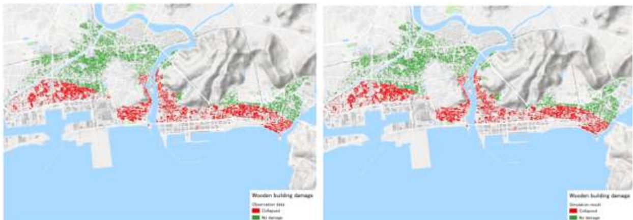
361 Fig. 9 Distributions of collapsed and non-collapsed buildings from field observation (left) and the 362 proposed method (right)
