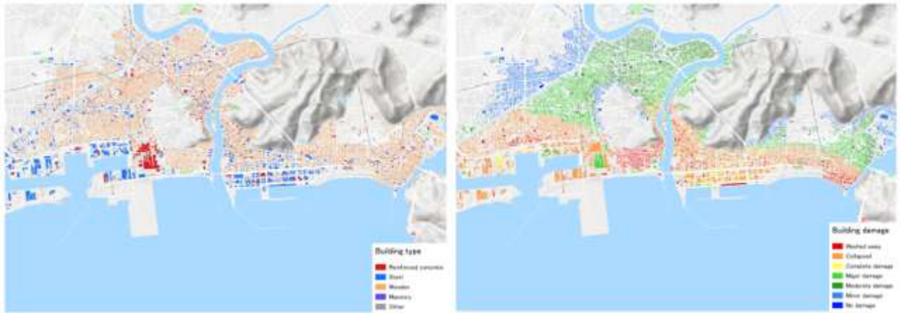
185 186 Fig.2 (Left) Distributions of building types and (Right) building damage levels.
