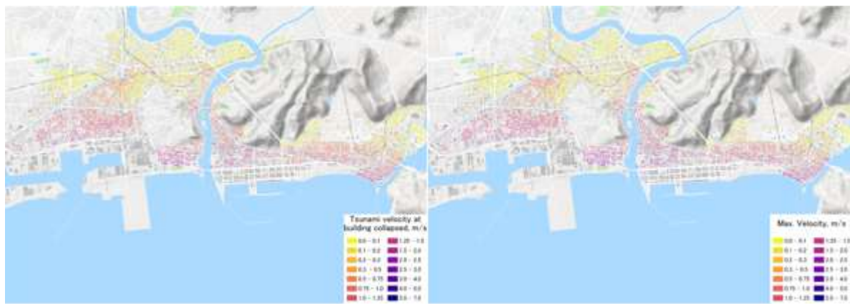
412 Fig. 11 Distribution of the simulated critical flow velocity (left) and the simulated maximum flow 413 velocity (right)
