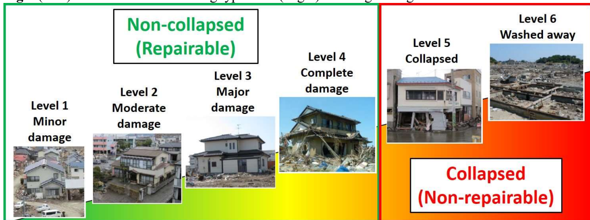
187 188 Fig. 3 Building damage levels and collapsed condition considered in this study (courtesy of MLIT, 189 2012).
