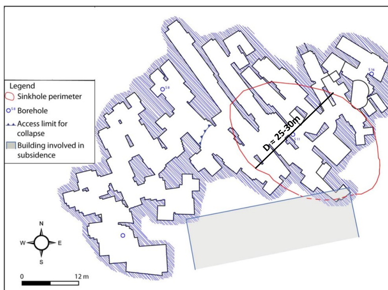
251 252 Figure 9. Plan of the Marsala underground quarry, with indication of the sinkhole area (adapted 253 after Vattano et al. 2013).
