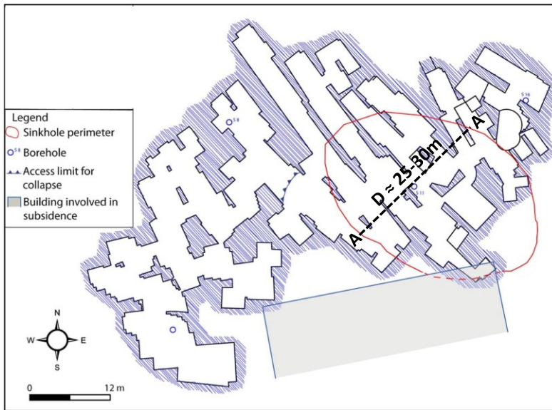
Figure 9. Plan of the Marsala underground quarry, with indication of the sinkhole area (adapted after Vattano et al. 2013).
