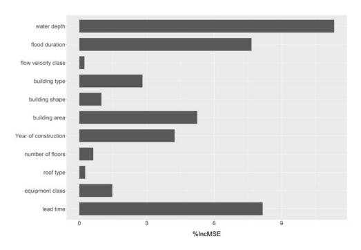
Figure 3: Random Forest variable importance for the estimation of building damage in the private households sector (n = 1610). 650 Importance measure is the Mean Square Error (%IncMSE).
