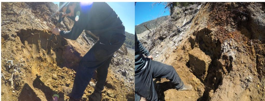
Figure 10: Extraction of an undisturbed soil sample
