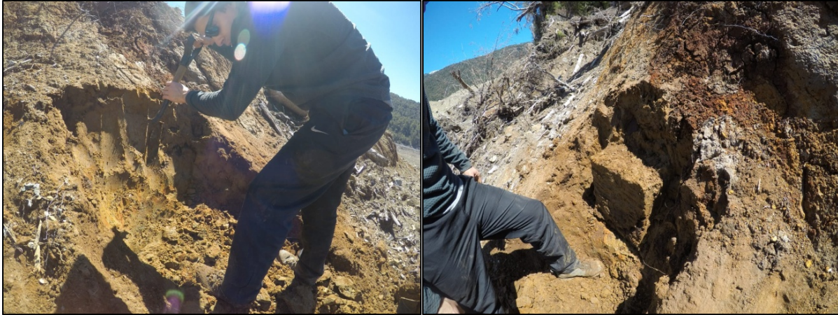
Figure 6: Extraction of an undisturbed soil sample
