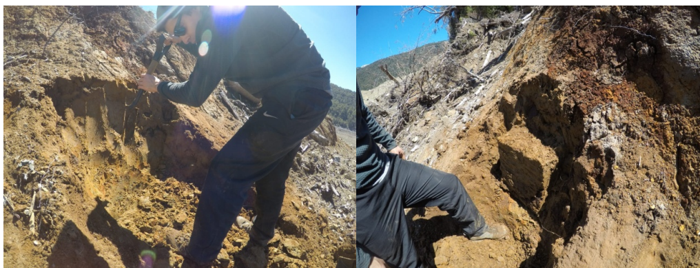
Figure 10: Extraction of an undisturbed soil sample
