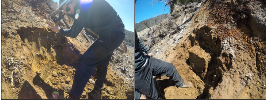
Figure 6: Extraction of an undisturbed soil sample
