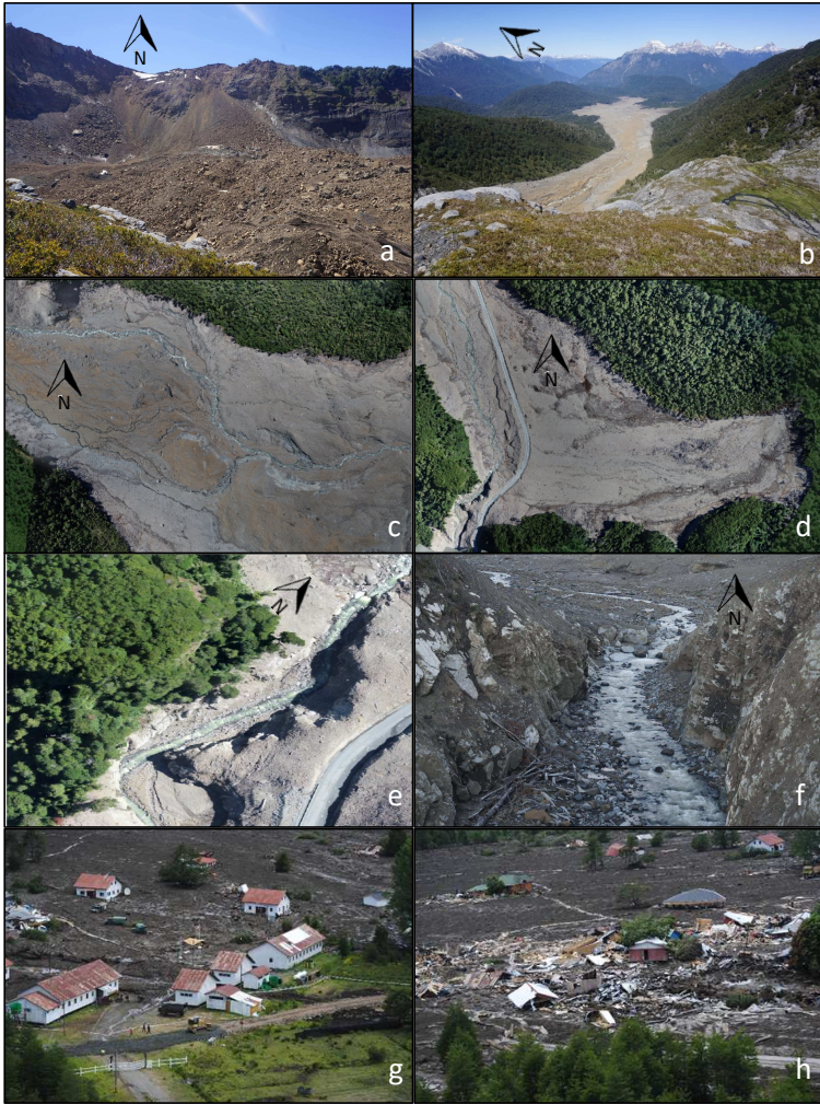
Figure 4: a) Area of slope failure slide and deposit; b) Channeled flow at the foothills; c and d) Aerial photo of non-channeled flood deposited in an old wetland captured with an InspireII UAV; e and f) photos of the channel in the last section before entering Villa Santa Lucia: left, captured with an InspireII UAV; right, picture of the channel facing downstream; h and i) Villa Santa Lucia after the mudflow (from Sernageomin (2018c)).
