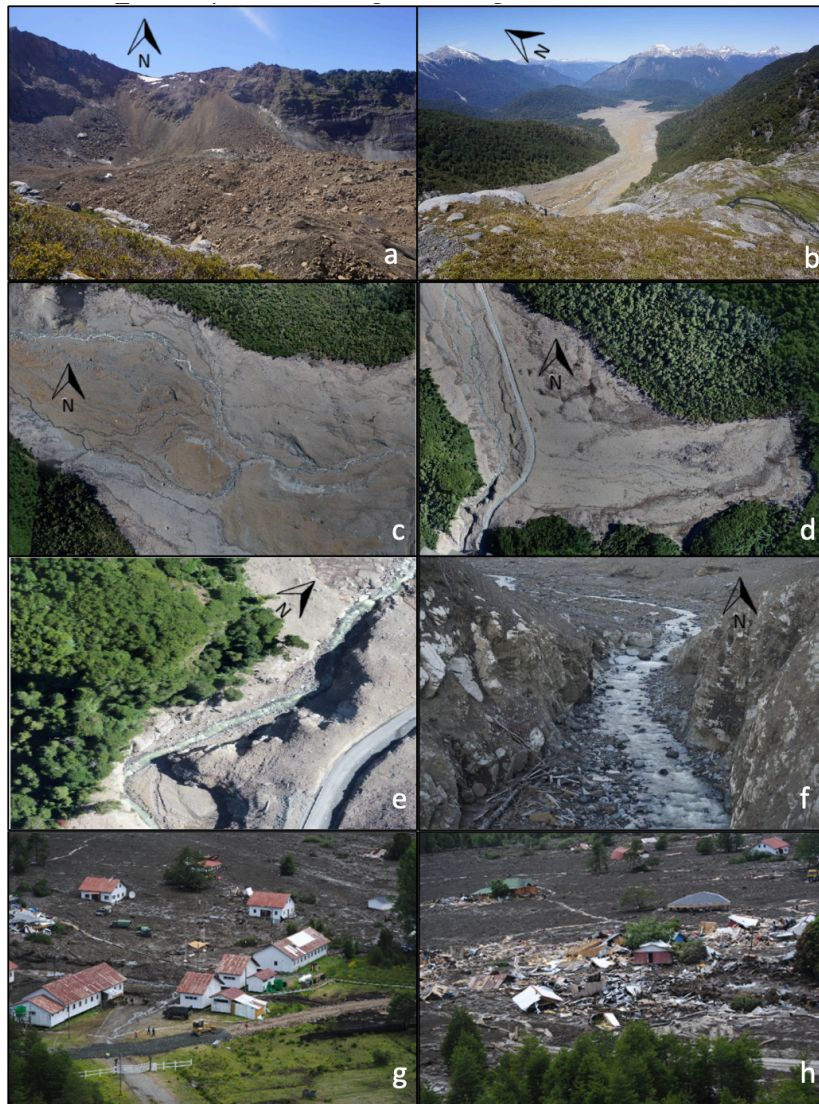
Figure 4: a) Area of slope failure slid and deposit; b) Channeled flow at the foothills; c and d) Aerial photo of non-channeled flood deposited in an old wetland captured with an InspireII UAV; e and f) Aerial photo of the channel in the last section before entering Villa Santa Lucia (left) captured with an InspireII UAV. Picture of the channel facing downstream (right); h and i) Villa Santa Lucia after the mudflow (From Sernageomin (2018c)).
