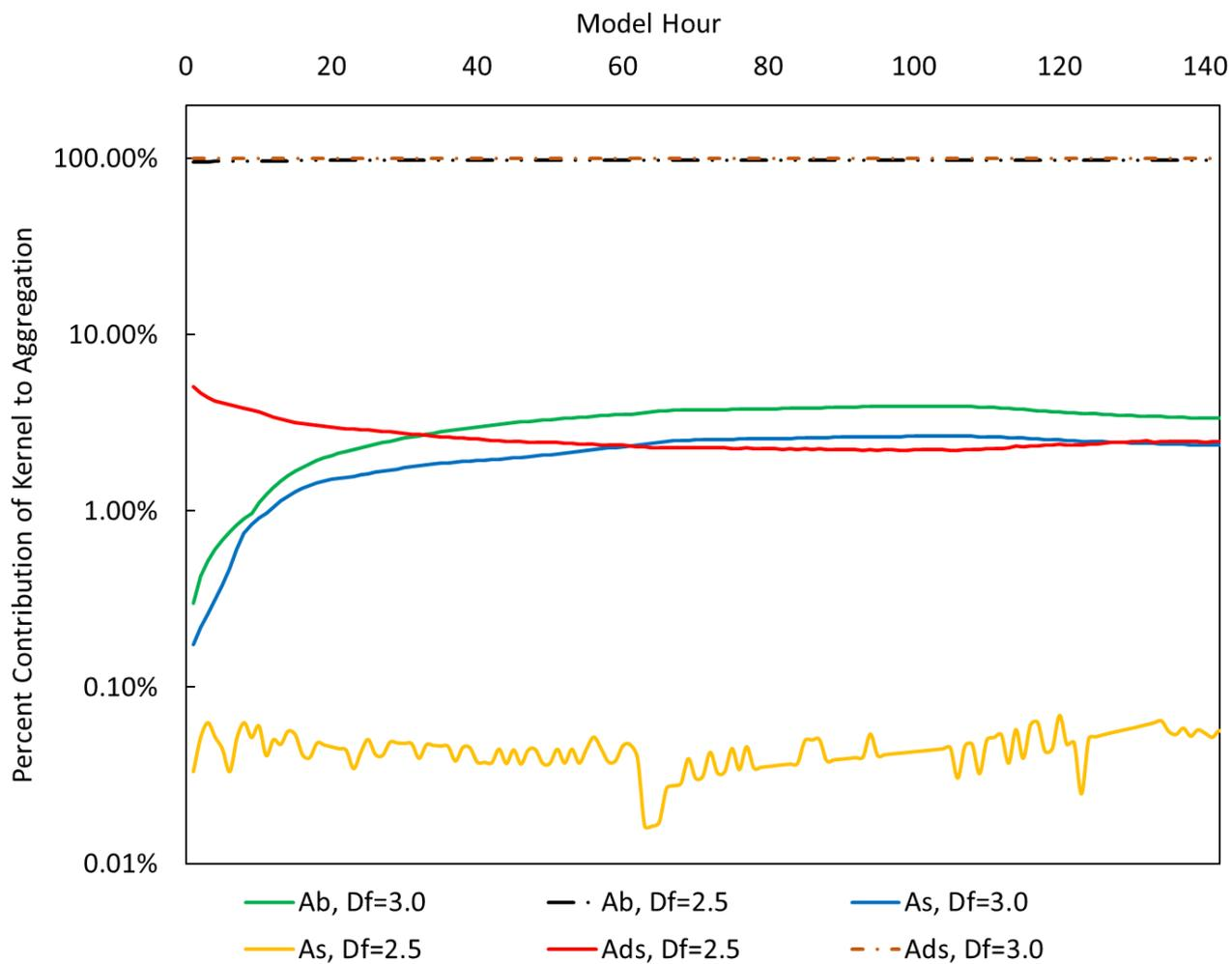
635 **Figure 5:** Percentage of aggregation rate for each collision kernel ( $A_B$  = Brownian,  $A_S$  = Shear,  $A_{DS}$  = Differential Sedimentation) when considering a hypothetical eruption on May 5<sup>th</sup>, beginning 00:00Z and ending 09:00Z, for two fractal dimensions,  $D_f = \{3.0, 2.5\}$ . Constant eruption rate =  $4 \times 10^6 \text{ kg s}^{-1}$ .
