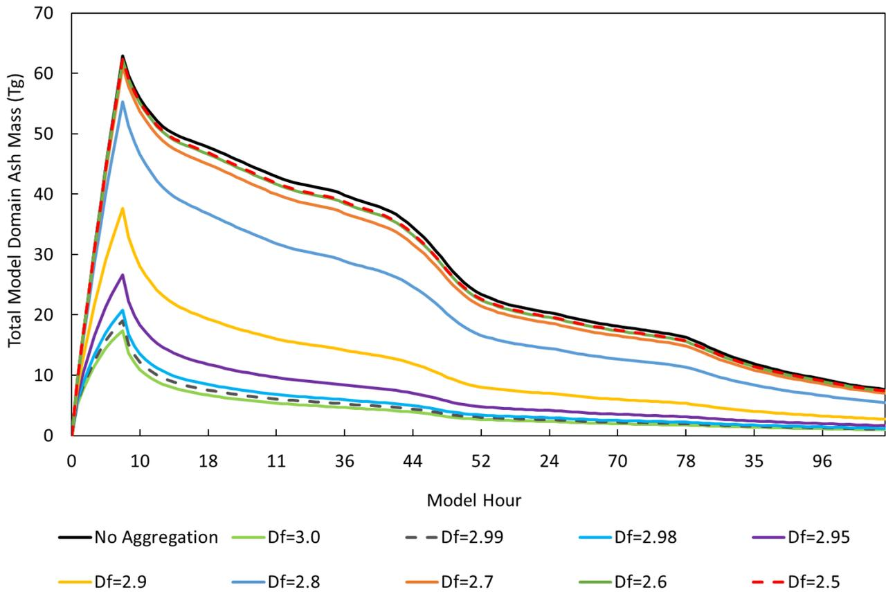
625 **Figure 3:** Change in total domain ash mass,  $T_g$ , for a hypothetical eruption on May 5<sup>th</sup>, beginning 00:00Z and ending 09:00Z, for a range of fractal dimensions,  $D_f = \{3.0, 2.99, 2.98, 2.95, 2.9, 2.8, 2.7, 2.6, 2.5\}$ . Constant eruption rate =  $4 \times 10^6 \text{ kg s}^{-1}$ .
