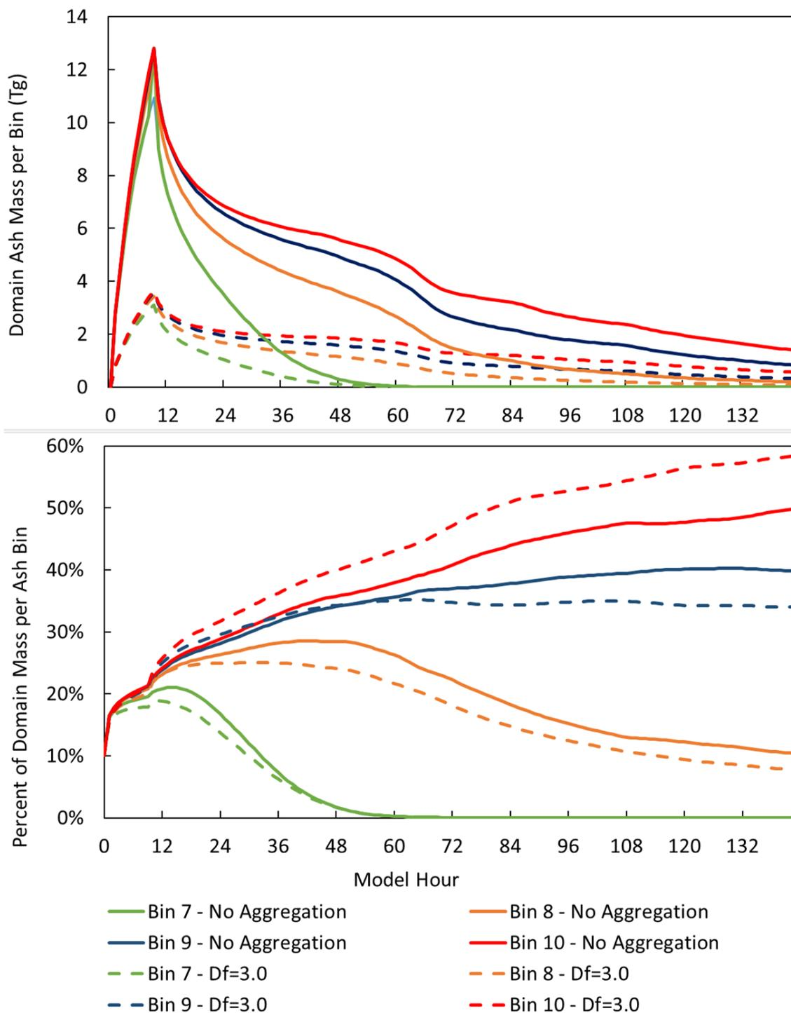
640 **Figure 6:** Total domain mass (A) and particle size distribution (B) of volcanic ash bins 7 to 10 when considering a hypothetical eruption on May 5<sup>th</sup>, beginning 00:00Z and ending 09:00Z, and a fractal dimensions,  $D_f = 3.0$ . Constant eruption rate =  $4 \times 10^6 \text{ kg s}^{-1}$ .
