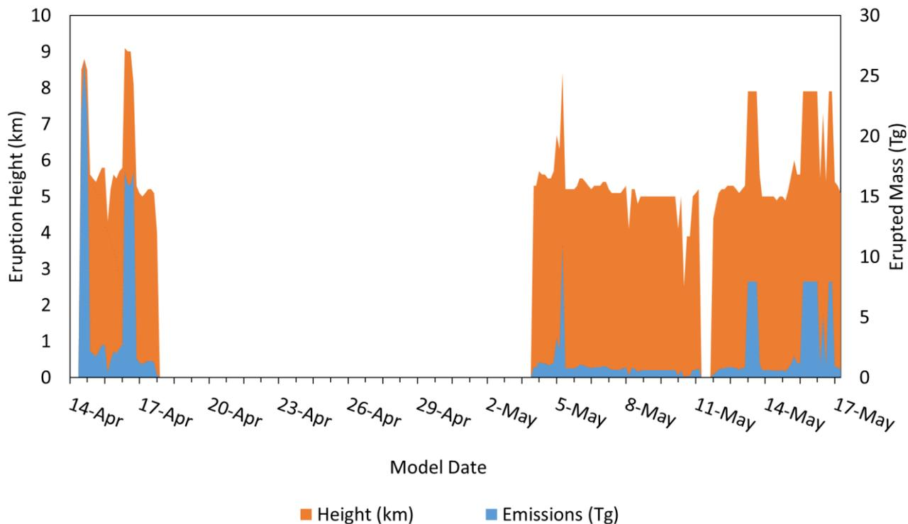
620 **Figure 2:** Three hourly plume heights (KM) ASL (orange, km) and emitted mass (blue, Tg) used in the WRF-Chem modeling simulations (volc\_d01.asc name list) for the eruption period April 12 until May 18, 2010. Values adapted from Hirtl et al., (2019) with dates as DD/MMM.
