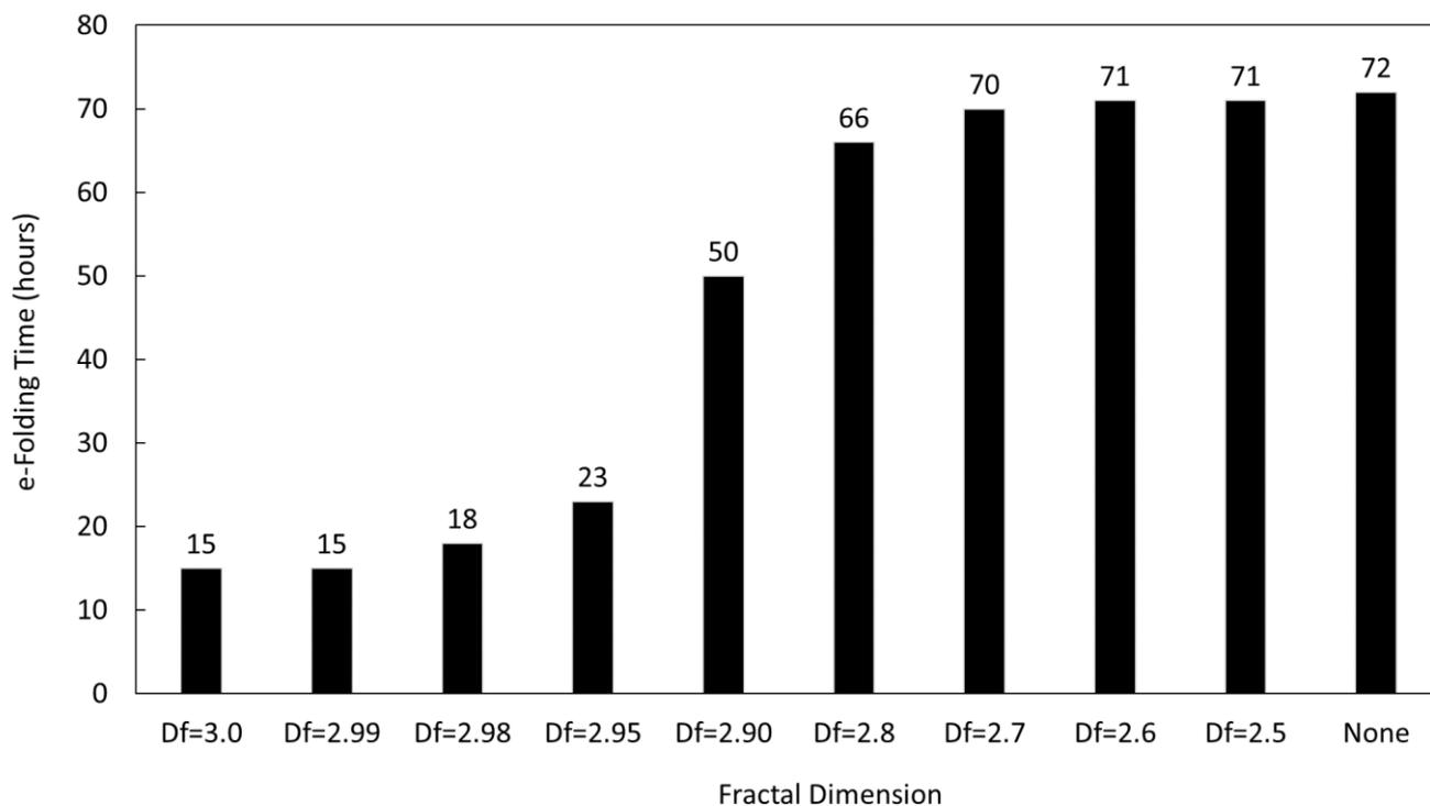
630 **Figure 4:** Volcanic ash e-folding time in hours for a hypothetical eruption on May 5<sup>th</sup>, beginning 00:00Z and ending 09:00Z, for a range of fractal dimensions,  $D_f = \{3.0, 2.99, 2.98, 2.95, 2.9, 2.8, 2.7, 2.6, 2.5\}$ . Constant eruption rate =  $4 \times 10^6 \text{ kg s}^{-1}$ .
