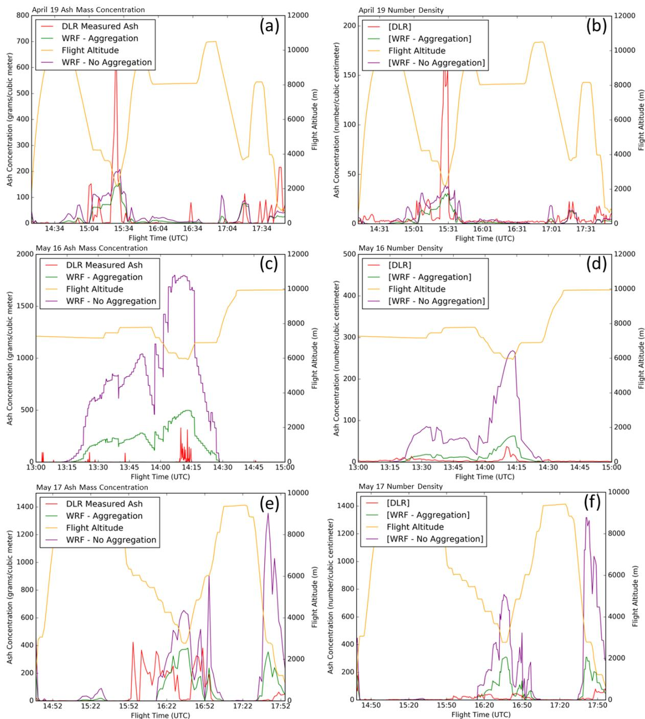
650 **Figure 8:** Comparisons of WRF-Chem model output to in situ mass concentrations (left panels) and particle numbers (right panels) observed by DLR during April 19 (A and B), May 15 (C and D) and May 17 (E and F), 2010 flights.
