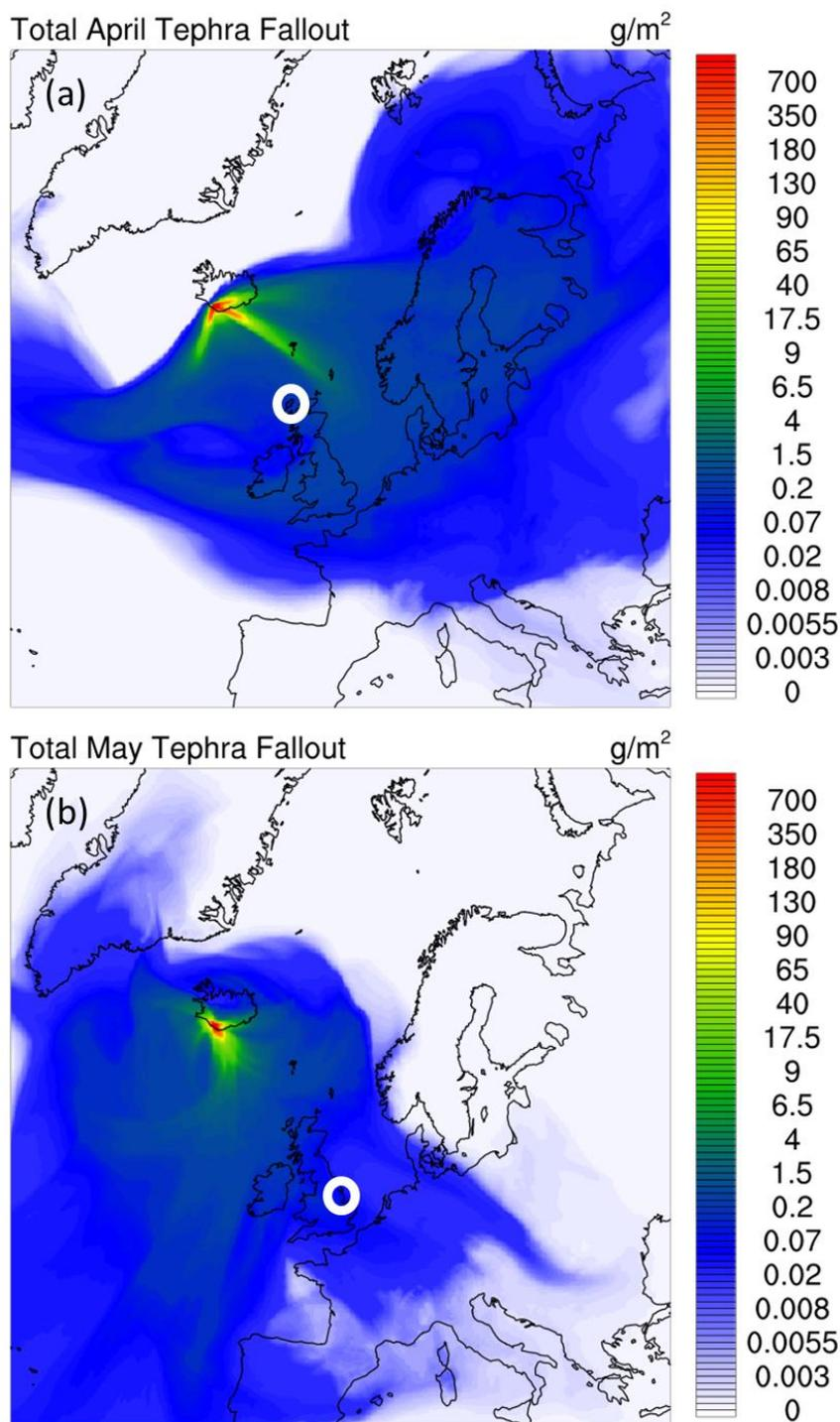
**Figure 9** Mass of tephra fallout deposited on model surface, lowest model level in WRF-Chem, for April (A,) and May (B) 2010 model simulations. White circle in (A) marks the Outer Hebrides and white circle in (B) marks Lincolnshire and Leicestershire, UK, corresponding to sample areas in Stevenson et al., (2012). Maximum domain fallout is  $52 \text{ Mg m}^{-2}$ .
