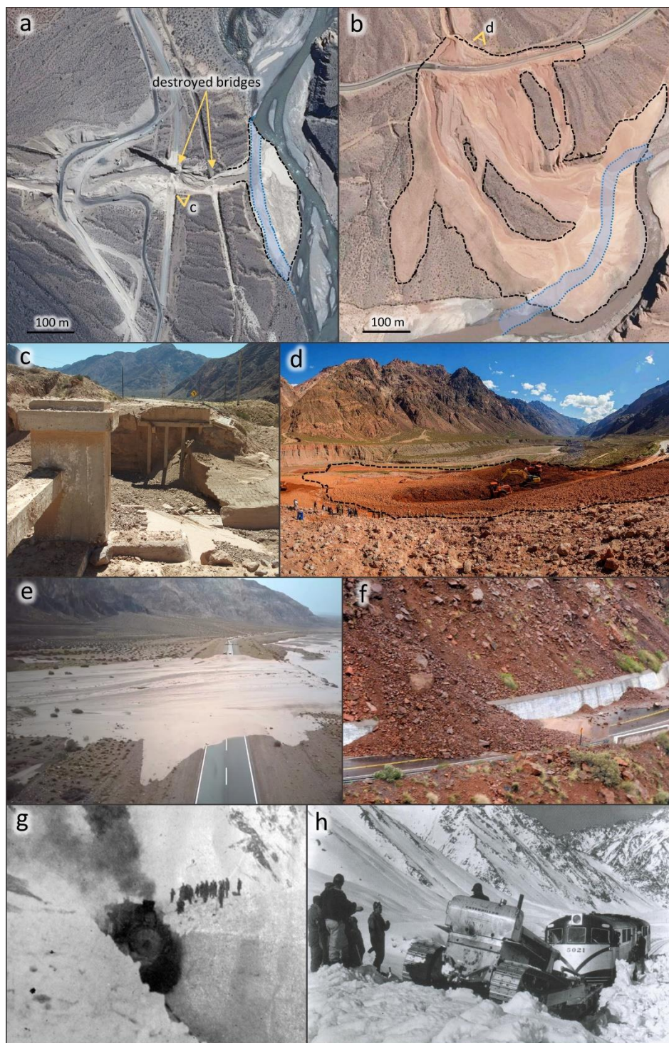
450 Figure 3: Pictures illustrating G-CHs in study area: (a,c) rainfall-driven debris flow occurred on 2 February 2016 in the E zone, (b,d) rainfall-driven debris flow occurred on 23 January 2016 in the E zone, (e) rainfall-driven debris flow occurred on 4 February 2018 in the E zone, (f) rainfall-driven debris falls occurred on 2 August 2013 in the E zone, (g,h) snow avalanches in the W zone.
