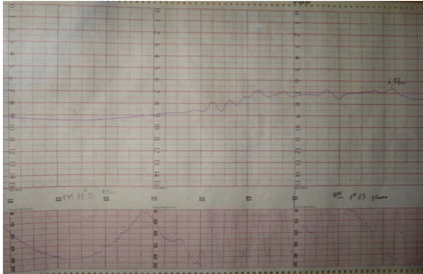
460 Figure 11 : Tide gauge record of the 1960 Chile tsunami in Nouméa (Chaleix station): original record (left) and digitized signal (right), total (in green) and detided (in blue).
