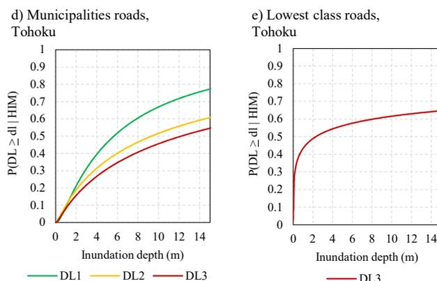
650 **Figure 18: Fragility functions for inundated State Roads (a), Main Local Roads (b), General Prefectural Roads (c), Municipalities Roads (d) and Lowest Class Roads (e) (as an indicator of construction type and materials) in Miyagi and Iwate prefectures following the 2011 Tohoku Earthquake and Tsunami, Japan.**
