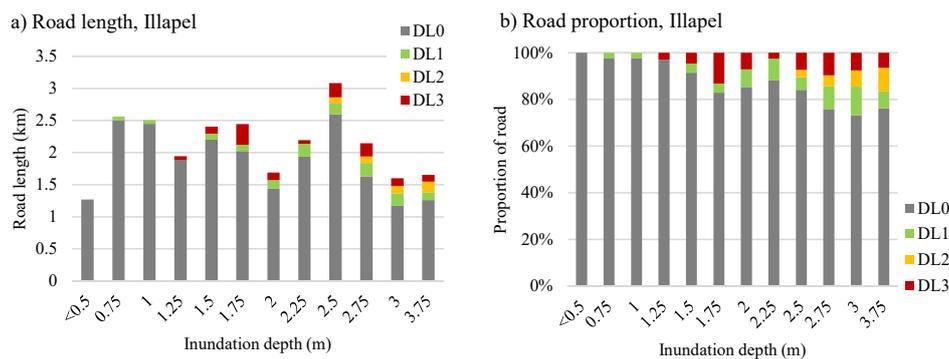
**Figure 3: Total length (a) and proportion (b) of exposed roads, by inundation depth, for the 2015 Illapel Earthquake and Tsunami**
