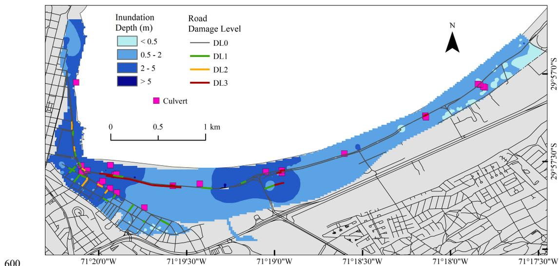
600 **Figure 2: Tsunami inundation, road damage level and culvert locations in Coquimbo, Chile following the 2015 Illapel Earthquake and Tsunami, © OpenStreetMap contributors 2015. Distributed under a Creative Commons BY-SA License.**
