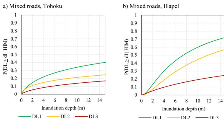
Figure 13: Fragility functions for mixed construction roads (a) for the 2011 Tohoku Earthquake and Tsunami, Japan and for mixed construction roads (b) for the 2015 Illapel Earthquake and Tsunami, Chile
