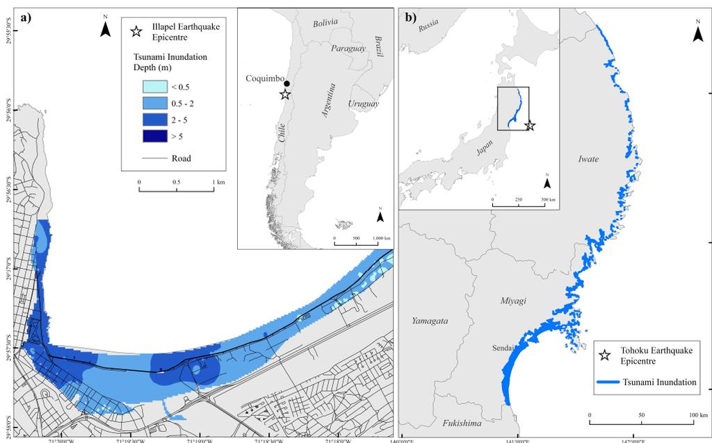
595 **Figure 1:** Tsunami inundation in Coquimbo for the 2015 Illapel tsunami, Chile (a), and in Miyagi and Iwate Prefectures for the 2011 Tohoku Tsunami, Japan (b), © OpenStreetMap contributors 2015. Distributed under a Creative Commons BY-SA License.
