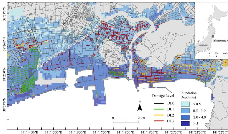
605 **Figure 4: Tsunami inundation and road damage in Ishinomaki, from the 2011 Tohoku Earthquake and Tsunami, Japan. Road-impact data modified from MLIT, 2012, © OpenStreetMap contributors 2015. Distributed under a Creative Commons BY-SA License.**
