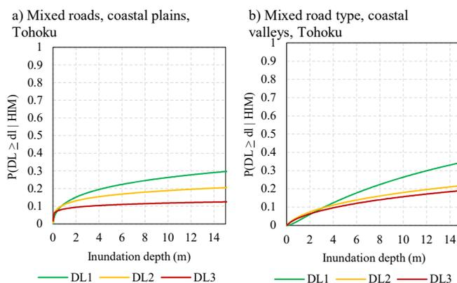
**Figure 19: Fragility functions for roads on coastal plains (a) and coastal valleys (b) for the 2011 Tohoku Earthquake and Tsunami, Japan**
