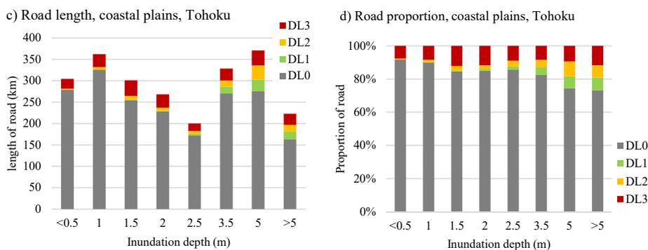
630 **Figure 12: Total length (a) and proportion (b) of exposed roads in a coastal valley topographic setting and total length (c) and proportion (d) of exposed roads in a coastal plain topographic setting, by inundation depth, for the 2011 Tohoku Earthquake and Tsunami**
