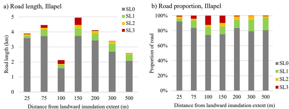
**Figure 10: Total length (a) and proportion (b) of exposed roads, considering levels of service, by distance from the landward inundation extent, for the 2015 Illapel Earthquake and Tsunami. Note SLU is not considered in analysis**
