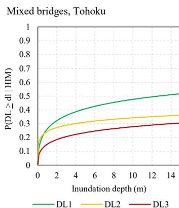
640 Figure 14: Fragility function for mixed construction road bridges for the 2011 Tohoku Earthquake and Tsunami, Japan
