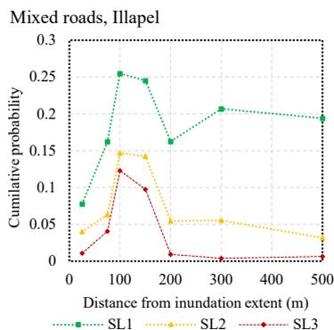
**Figure 17: Cumulative probability plot of road service levels compared with a distance from the in-land extent of tsunami inundation (as an indication of debris density sorting) for the 2015 Illapel Tsunami, Coquimbo, Chile.**
