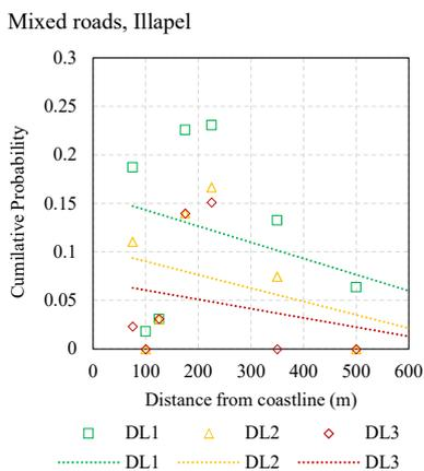
645 Figure 16: Linear best fit probability of reaching or exceeding a given damage level, by distance from coastline (as a proxy for inundation energy, for the 2015 Illapel Tsunami, Coquimbo, Chile
