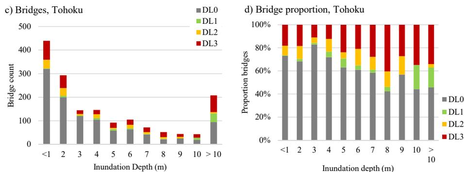
**Figure 5:** Total length (a) and proportion (b) of exposed roads and number (c) and proportion (d) of exposed bridges, by inundation depth, in Miyagi and Iwate Prefectures for the 2011 Tohoku Earthquake and Tsunami
