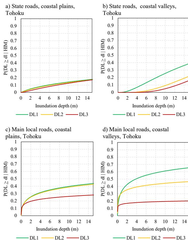
655 **Figure 20: Fragility functions for road State Roads on coastal plains (a) and coastal valleys (b), and for Main Local Roads on coastal plains (c) and coastal valleys (d) for the 2011 Tohoku Earthquake and Tsunami, Japan**
