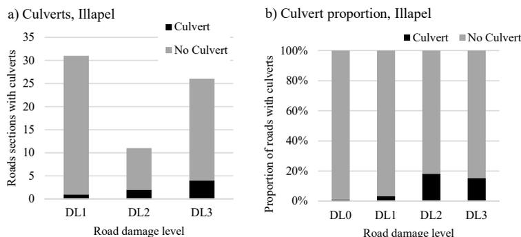
615 **Figure 7: Number (a) and proportion (b) of road sections with or without a culvert, by damage level, for the 2015 Illapel Earthquake and Tsunami**
