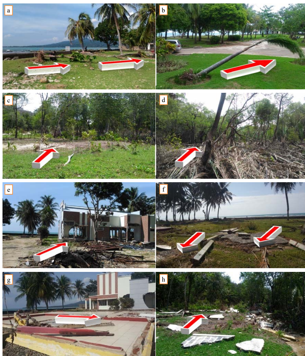
Figure 3: Evidence of tsunami direction. Arrows show the direction of tsunami flow on the ground surfaces.
