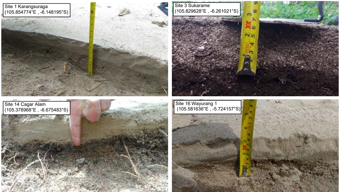
Figure 5. Tsunami sediment deposit, test pits were made to measure the deposit thickness.
