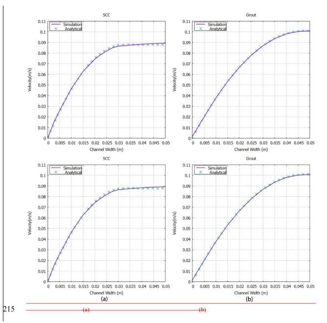
Figure 2: Comparison of velocity variation between analytical solutions (Gopala et al., 2011) and numerical results simulated in two parallel plates based on different rheological parameters. i.e. (a) SCC and (b) Grout.
