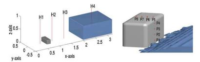
Figure 3: Measurement positions for water heights and pressures in the dam-break experiment. (from Kleefsman (Kleefsman et al., 2005)). P1 to P8 are pressure probes, and H1 to H4 are height probes.
