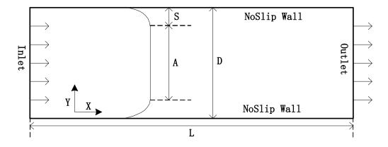
Figure 1: Schematic of the flow between parallel plates.
