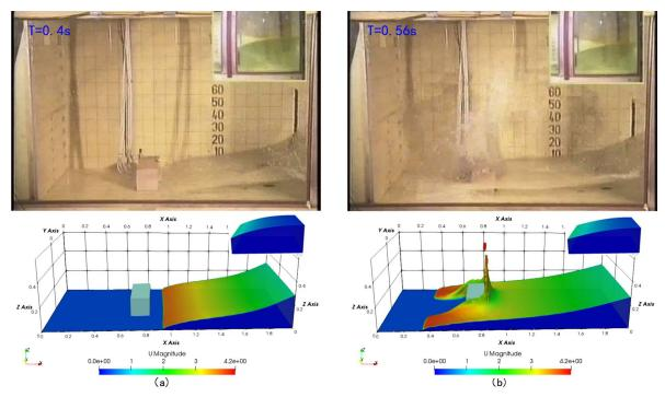
Figure 4: Screenshots of the simulation compared with the experiment (Kleefsman et al., 2005) at t = 0.4 s (a) and t = 0.56 s (b). The color map of the simulation results is mapped by velocity characteristics.
