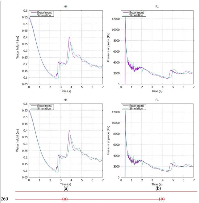
Figure 5: Comparison of vertical water heights in reservoir at probe H4 (a) and <u>the</u> characteristic curve of pressure changing with time at probe P1 (b) between experimental data and simulation results.
