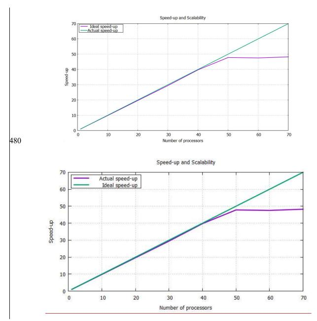
Figure 16: Parallel speedup with different numbers of processors. The green line is the ideal speedup, and the purple line is the actual speedup.
