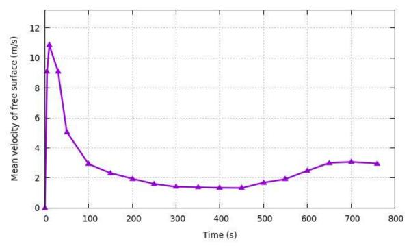
Figure 15: Average velocity time-history for the free surface simulated of the A'xi dam failure.
