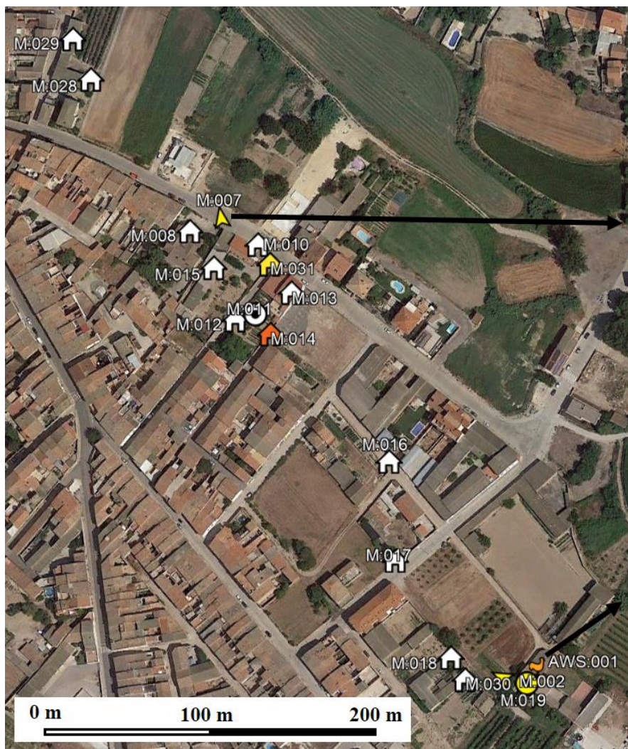
Figure 7. Data location map and two examples of recorded information from the 21 March 2012 EF1 Ivars d'Urgell (Catalonia) tornado track. Map symbols indicate locations of AWS (orange weathervane), damage in man-made structures (house icon) and fallen trees or damaged vegetation elements (arrow and circle icon if no direction is available, respectively). Icon colours indicate damage intensity using the EF-scale: EF0 (yellow), EF1 (orange) and unrated (white). The background orthophoto is from the Institut Cartogràfic i Geològic de Catalunya (ICGC), http://www.icc.cat (last access: September 2019), under a CC BY 4.0 license.
