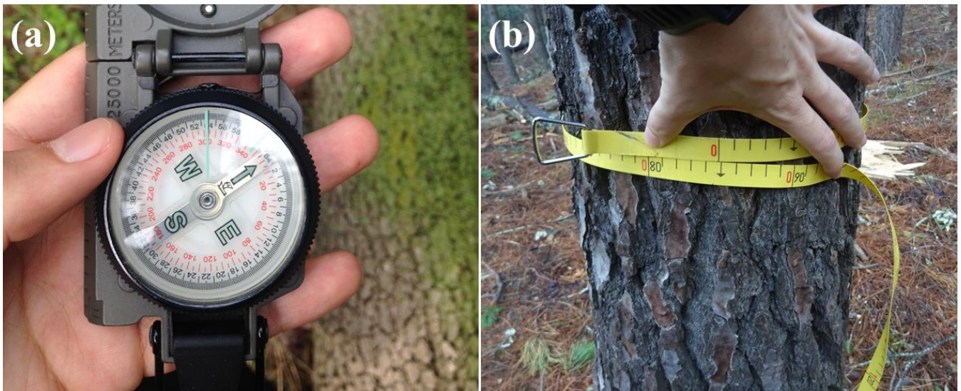
Figure 5. (a) Measure of the fall direction of a tree and (b) measure of trunk diameter during the damage survey of an EF1 tornado on 13 October 2016 in Llinars del Vallès (Catalonia) and an EF2 tornado on 7 January 2018 in Darnius (Catalonia), respectively (Author: Oriol Rodríguez).
