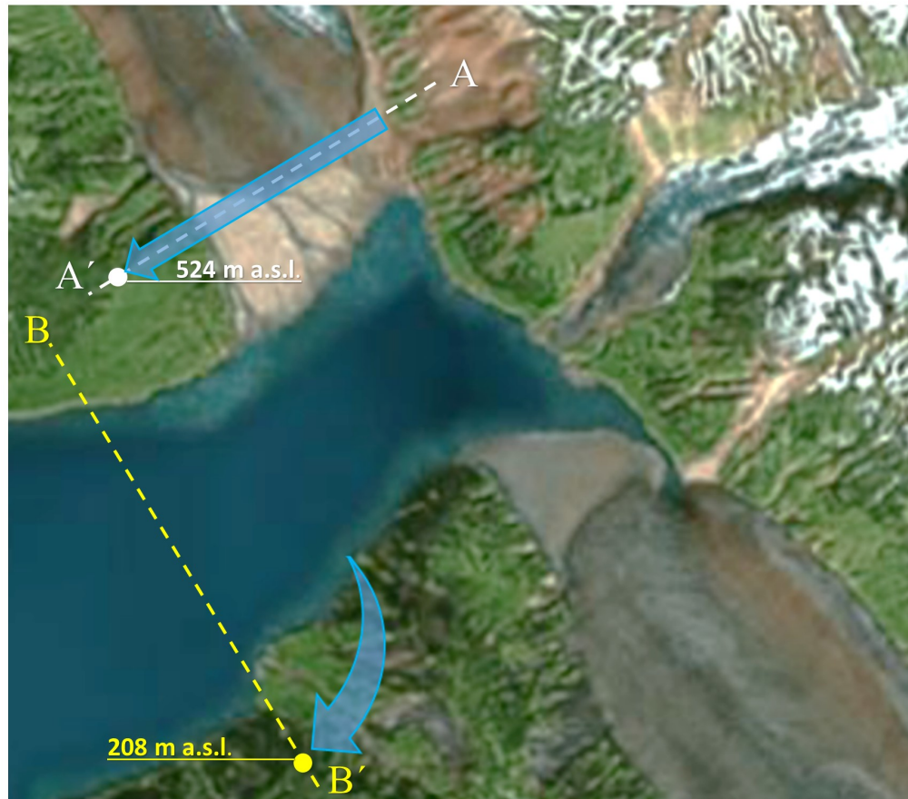
Fig. 1. Sections where the two maximum run up heights are calculated. The light blue arrows show the direction of the wave flowing upon the topographic surface.
