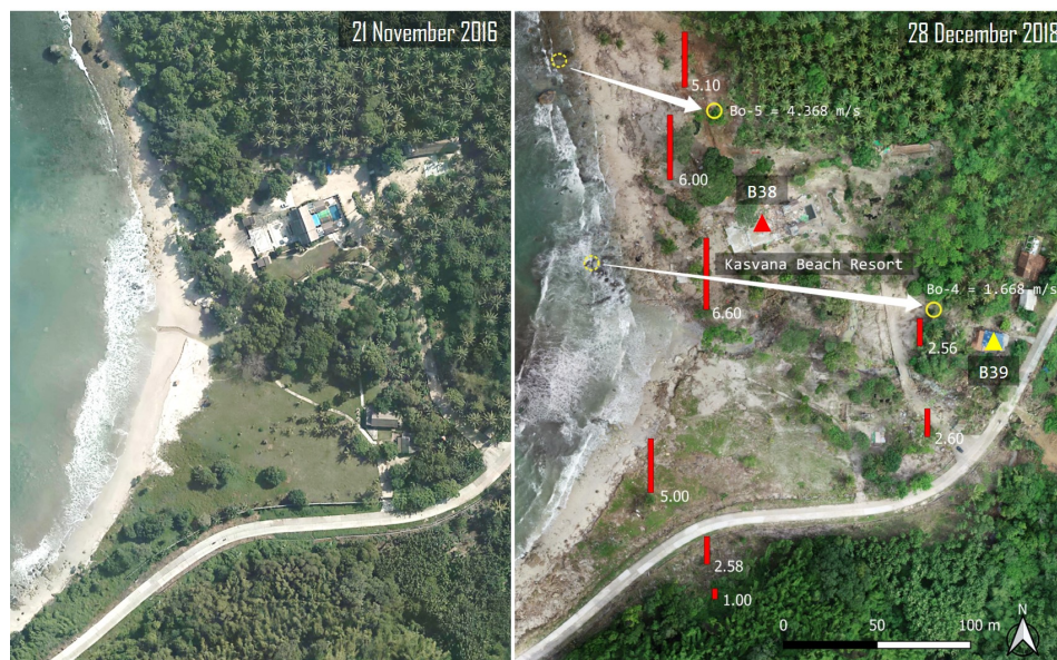
Fig. 7. The land destruction and flow depth distribution in Cipenyu Beach, Banten. Left hand-side photo is a google earth image captured before the tsunami (from © Google Earth). Right hand-side photo is an aerial view captured by drone on December 29, 2018.
