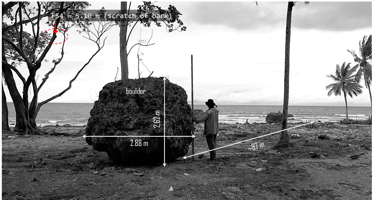
Fig. 8. The largest boulder found in Cipenyu Beach of Banten was transported about 87 m from its original place. An arrow shows the estimated transport direction of the boulder with an estimated velocity of 4.37 m/s.; captured on December 28, 2018.
