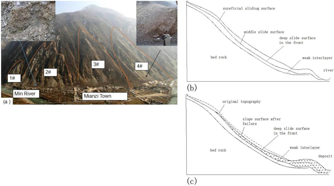
**Fig. 15** Photograph and schematic of the **rock** avalanche at Mengjiacao, Mianzi town, Wenchuan, Sichuan, China: (a) photograph at Mengjiacao; (b) schematic of toppling rockfall before failure; and (c) schematic of toppling rockfall after failure.
