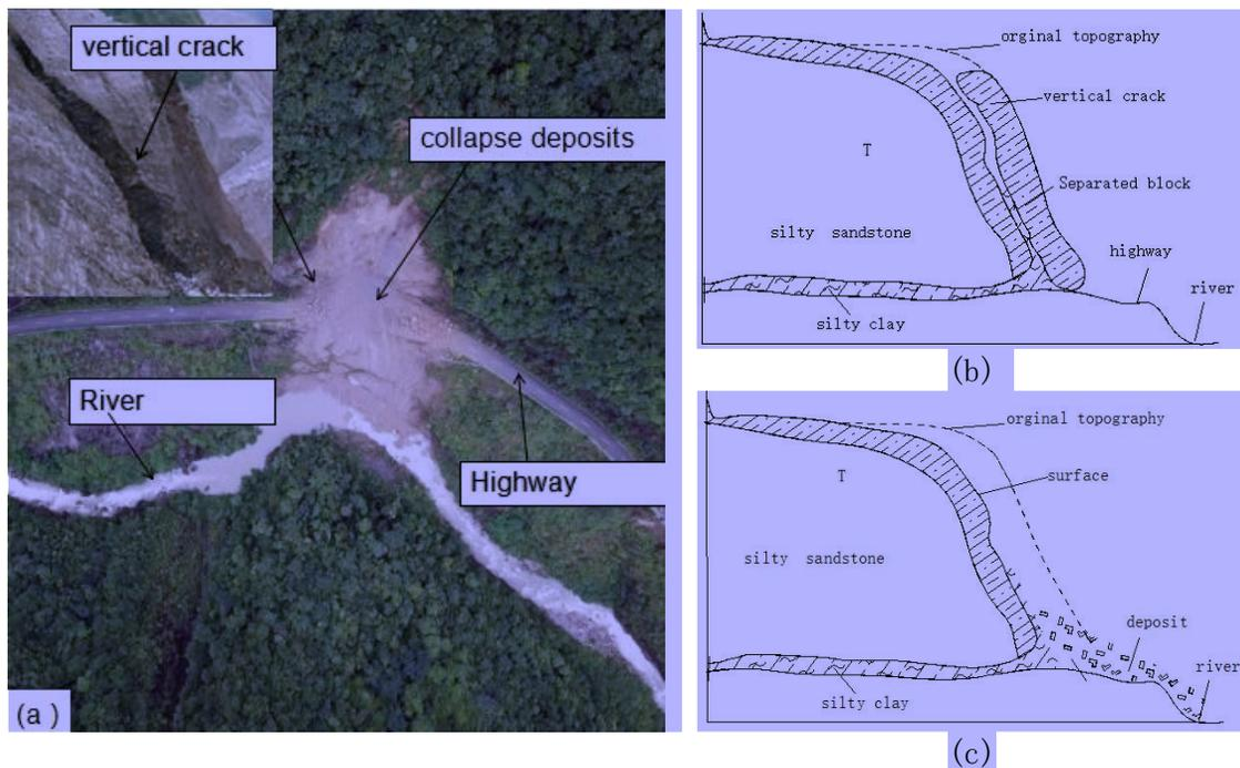
**Fig. 10 Aerial photograph and schematic of crack-slide rockfall in Jiguan Mountain, Chongzhou city, Sichuan, China, in 2018: (a) aerial photograph of Jiguan Mountain; (b) schematic of loose deposits before failure; and (c) schematic of the crack-slide rockfall.**
