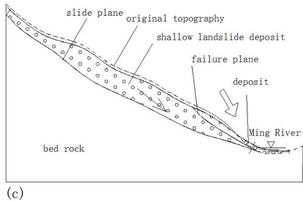
**Fig. 13 Schematic and photograph of bank erosion in Rope bridge/Soqiao village, Wenchuan County, Sichuan Province, China, in 2014: (a) photograph of gully erosion of the bank deposit; (b) schematic of deposits before the failure; and (c) schematic of deposits after the failure.**
