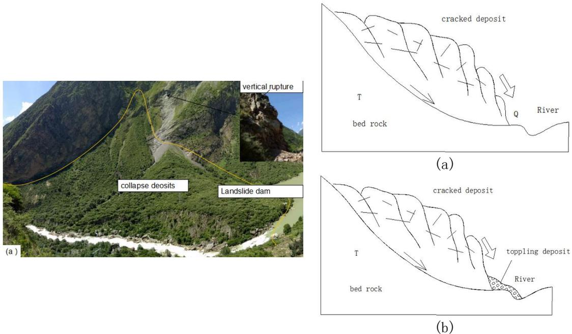
**Fig. 11 Aerial photograph and schematic of toppling rockfall at Yinping, Mao County, Sichuan, China: (a) aerial photograph at Yinping; (b) schematic of toppling rockfall before failure; and (c) schematic of toppling rockfall after failure.**
