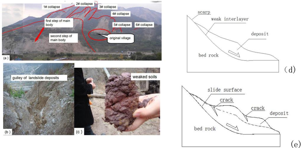
**Fig. 6** The landslide that occurred at Fenghuang Mountain, Sichuan, China, in 2011: (a) image of Fenghuang Mountain landslide; (b) Gully at the trailing edge of a landslide; (c) soft crushed soil from drilling; (d) Schematic of loose deposits before failure; and (e) Schematic of loose deposits after failure.
