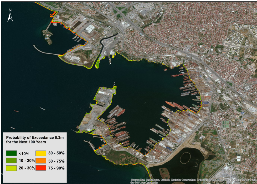
Figure 8: Probabilistic Tsunami Inundation Maps for Tuzla Study Domain representing the Probability of Exceedance of 0.3 m Inundation Depth within the Next 50 and 100 Years. Change of colors from green to red represents the increasing probability of exceedance (created using ArcMap Version 10.5).
