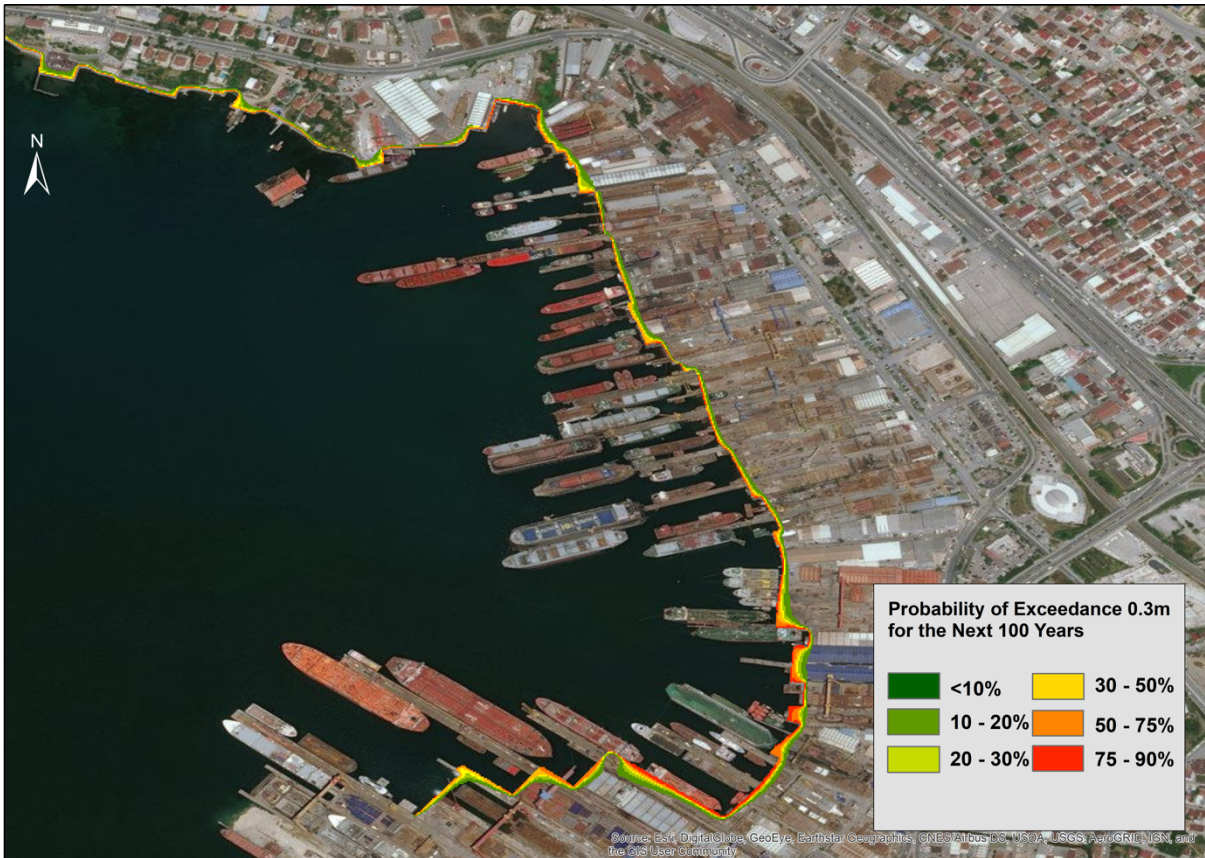
420 Figure 11: Probabilistic Tsunami Inundation Maps of Shipyard Area in Tuzla Study Domain representing the Probability of Exceedance of 0.3 m Inundation Depth for the Next 50 and 100 Years. Change of colors from green to red represents the increasing probability of exceedance (created using ArcMap Version 10.5).
