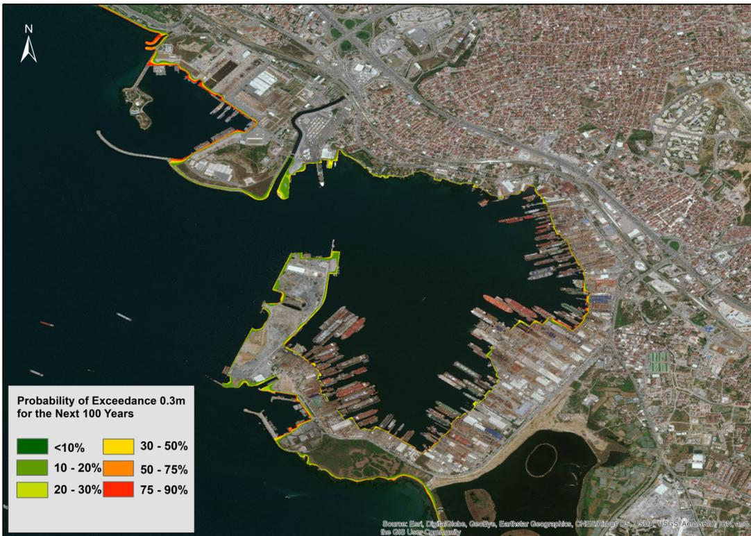
**Figure 7: Probabilistic Tsunami Inundation Maps for Tuzla Study Domain representing the Probability of Exceedance of 0.3 m Inundation Depth within the Next 50 and 100 Years. Change of colors from green to red represents the increasing of probability of exceedance (created using ArcMap Version 10.5).**
