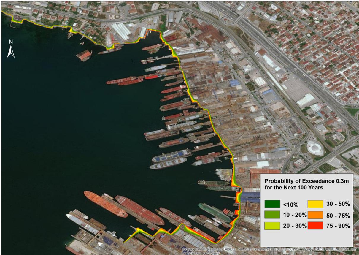
**Figure 10: Probabilistic Tsunami Inundation Maps of Shipyard Area in Tuzla Study Domain representing the Probability of Exceedance of 0.3 m Inundation Depth for the Next 50 and 100 Years. Change of colors from green to red represents the increasing of probability of exceedance (created using ArcMap Version 10.5).**
