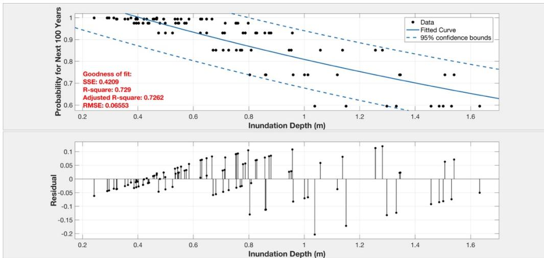
**Figure 6: Probabilities of Exceedance Corresponding to Maximum Water Surface Elevation, Minimum Water Surface Elevation and Inundation Depth for the next 100 years. Black dots represent the probability of exceedance of tsunami hydrodynamic parameter for each event in the catalog. Blue line is the best fit curve to the data and dashed blue line is the 95% confidence boundary of fitted curve. Residual of the fit is represented for each probability curves.**
