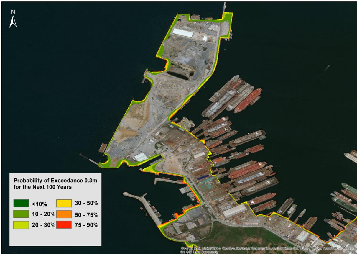
395 **Figure 9: Probabilistic Tsunami Inundation Maps for the Southern Part of Tuzla Study Domain representing the Probability of Exceedance of 0.3 m Inundation Depth for the Next 50 and 100 Years. Change of colors from green to red represents the increasing of probability of exceedance (created using ArcMap Version 10.5).**
