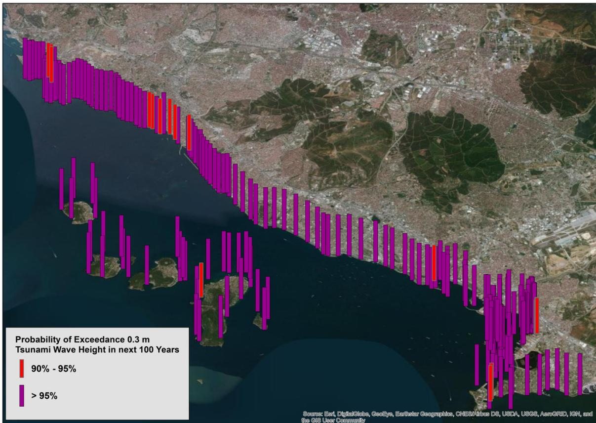
430 **Figure 11: Probability of Exceedance of 0.3 m Tsunami Wave Height within the next 50 and 100 years at Synthetic Gauge Points**
