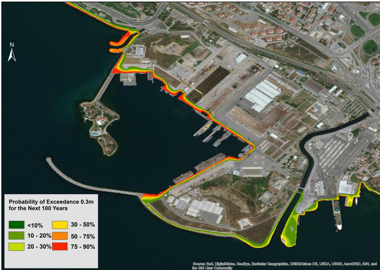
**Figure 8: Probabilistic Tsunami Inundation Maps of Northern Part of Tuzla Study Domain representing the Probability of Exceedance of 0.3 m Inundation Depth for the Next 50 and 100 Years. Change of colors from green to red represents the increasing of probability of exceedance (created using ArcMap Version 10.5).**
