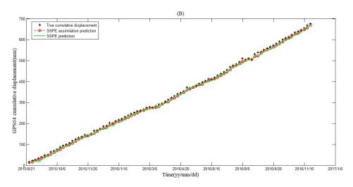
Fig. 7. Figure 9. The cumulative displacement prediction of (B)station GPS04
