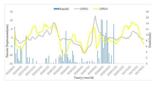
$\textbf{Fig. 3.} \ \ \textbf{Figure 7.} \ \ \textbf{The periodic term displacement combined with rainfall data in GPS03 and GPS04}$
