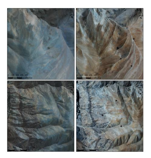
**Figure 3.** Optical imagery retrieved from Planet Team (2017) before and after March 2015 storm. Left images are before the March 2015 storm and right images are after. Arrows indicates different physical evidence of erosion processes due to the event and gully presence after March 2015 storm. The general color tone change merely indicates different sun illumination.
