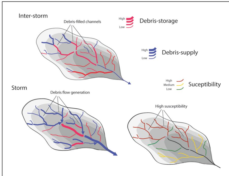
**Figure 10.** Conceptual model of the relation between hydraulic capacity during the intense long-lived rainfalls of an extraordinary storm and debris storage at previous time span that explain different levels of debris flow susceptibility depending on catchment topography.
