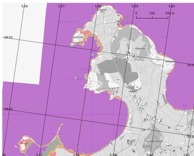
**Figure 7.** Stack of inundation maps covering Randaberg located on soft moraine in the southwest of Norway. Violet: Present MHW. Green: MHW for 2090 (0.79 m above present MHW). Orange: present 200-year storm surge (0.99 m above present MHW). Red: 200-year storm surge for 2090 (1.78 m above present MHW).
