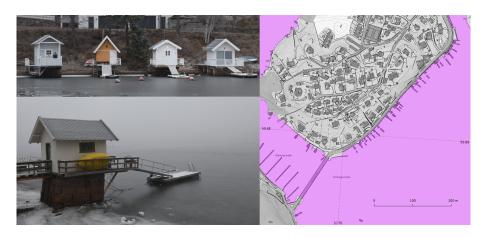
**Figure 2.** Buildings on piers or pillars above the water surface, like here at Ormøya close to Oslo, are erroneously mapped as flooded for present MHW (violet). Photo: Kristian Breili.
