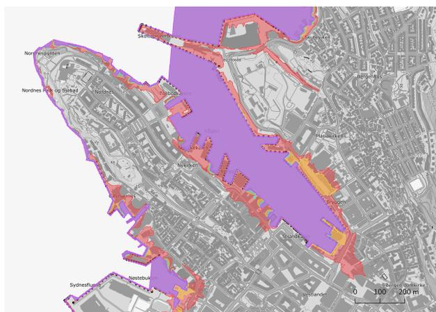
**Figure 9.** Stack of inundation maps indicating areas affected by coastal flooding in Bergen. Violet: Present MHW. Green: MHW at 2090 (0.71 m above present MHW). Orange: present 200-year storm surge (0.96 m above present MHW). Red: 200-year storm surge for 2090 (1.68 m above present MHW).
