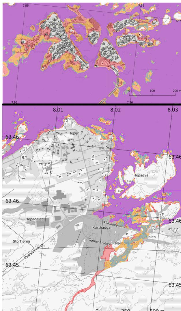
**Figure 4.** Stack of inundation maps covering the northern part of the island Smøla (lower panel) and the fishing village of Veiholmen (upper panel) located on the strandflat in the middle of Norway. Violet: Present MHW. Green: MHW for 2090 (0.74 m above present MHW). Orange: Present 200-year storm surge (1.29 m above present MHW). Red: 200-year storm surge for 2090 (2.03 m above present MHW).
