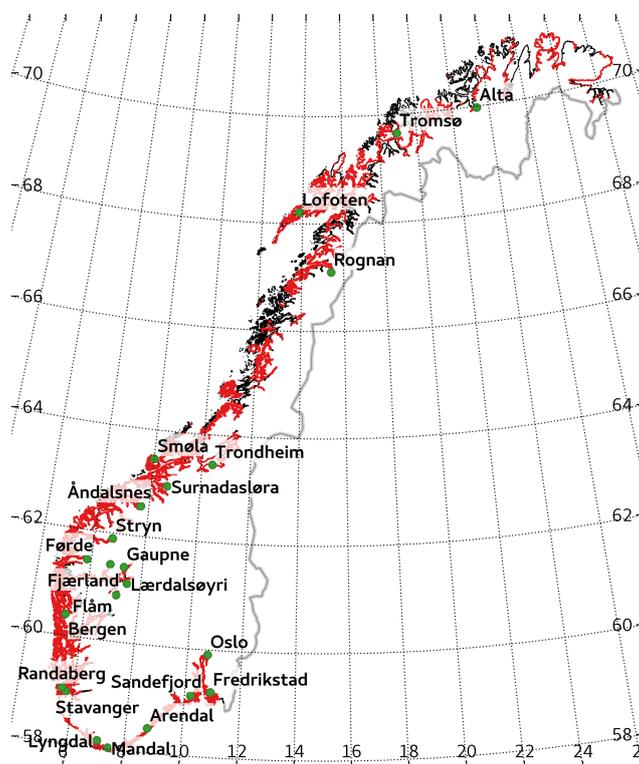
**Figure 3.** Red lines indicate areas covered by the inundation maps per December 2018. Information for all water levels is not available for all mapped zones due to a lack of knowledge on ocean tides for parts of the coast. In these zones, only the storm-surge return heights can be calculated because they are not referenced to MHW. The green markers indicate locations discussed in the text.
