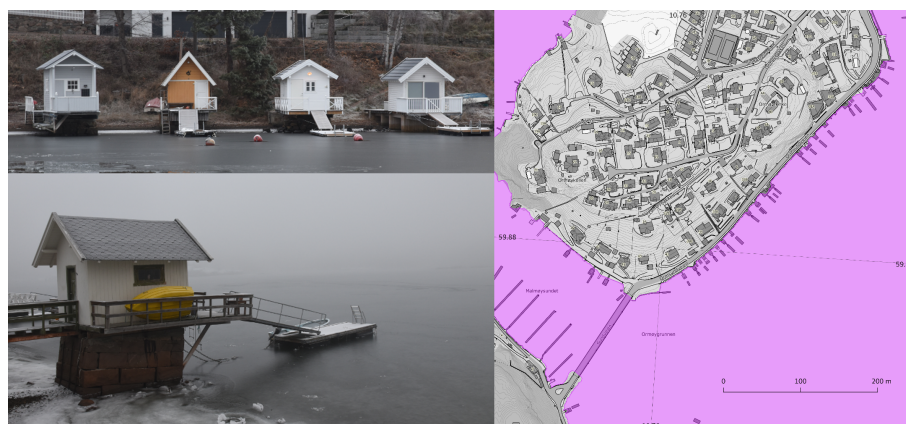
Figure 2. Buildings on piers or pillars above the water surface, like here at Ormøya close to Oslo, are erroneously mapped as flooded for present MHW (violet). Photo: Kristian Breili.
