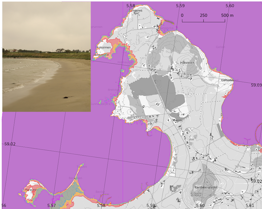
Figure 3. Stack of inundation maps covering Randaberg located on soft moraine in the southwest of Norway. Violet: Present MHW. Green: MHW for 2090 (0.79 m above present MHW). Orange: present 200-year storm surge (0.99 m above present MHW). Red: 200-year storm surge for 2090 (1.78 m above present MHW). Inset: Soft sand dunes at Sandestranda close to Randaberg. Photo: Oda R. Ravndal.
