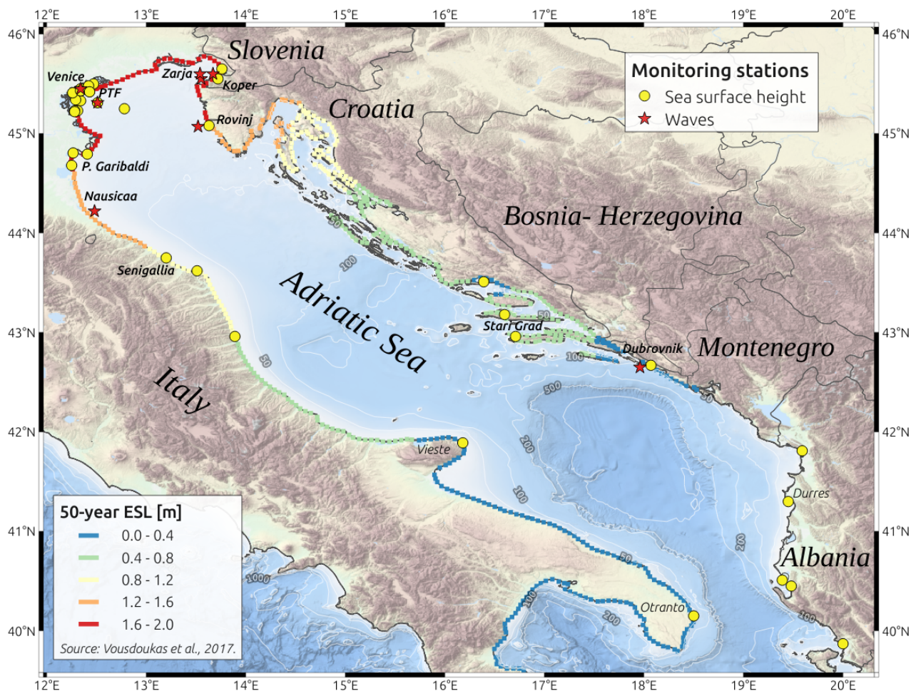
Figure 1. Bathymetry of the Adriatic Sea with monitoring stations for sea surface height (yellow dots) and waves (red stars). The 50-year extreme sea levels (ESL) from Vousdoukas et al. (2017) are also reported. Background: EMODnet bathymetry (EMODnet Bathymetry Consortium, 2018).
