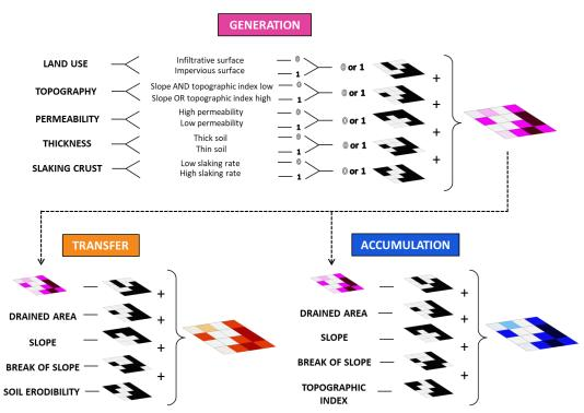
Figure 1: Scheme of the IRIP model presenting the various indicators computed to produce the susceptibility maps to runoff generation (top), transfer (bottom left) and accumulation (bottom right).
