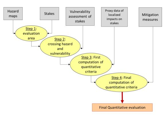
Figure 2: Scheme of the evaluation methodology to assess the relevance of susceptibility maps to runoff, using localized runoffrelated impacts proxy data.
