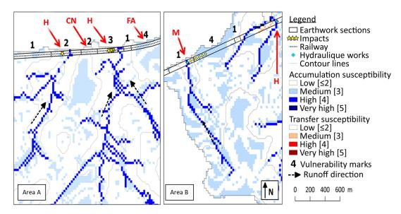
Figure 7: Illustration of the evaluation area and of the building of contingency tables on two sub-areas. The evaluation area is the buffer (black contours) along the railway line (black dotted line). The latter is divided into sections (earthwork sections) to which a
