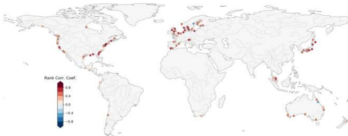
Figure S4: Spearman's rank correlation between the storm surge annual maxima occurrence obtained from the model and from the observations.
