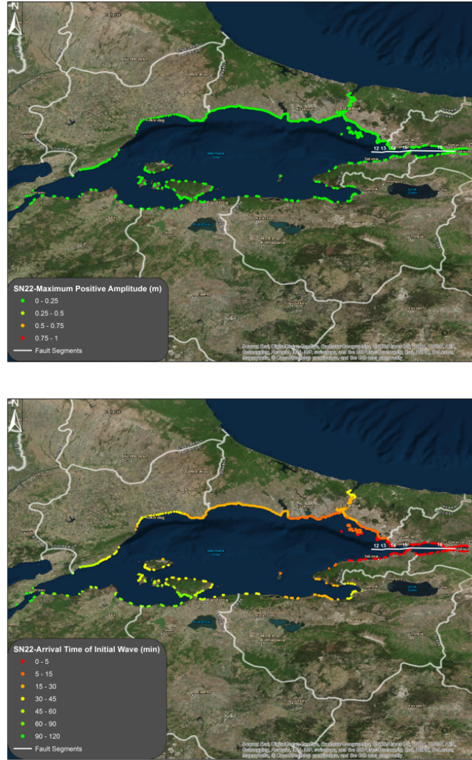
Figure 43: Distribution of maximum wave amplitudes and arrival time of first wave along the coasts of Marmara Sea regarding to scenario SN22. The maximum wave amplitudes calculated for this scenario are less than 25cm in entire Marmara Sea.
