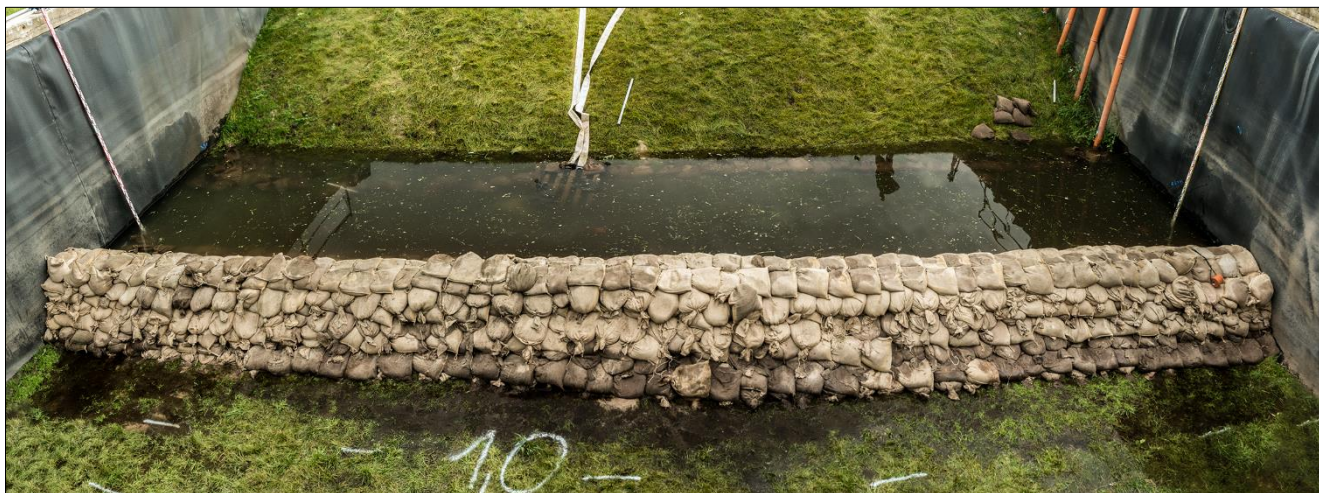
5 Figure 6: Sandbag dam in the IWA test facility.
