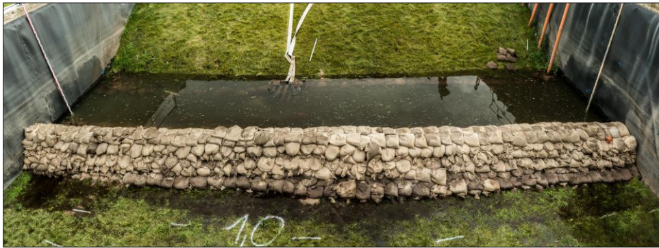
Figure 6: Sandbag dam in the IWA test facility.
