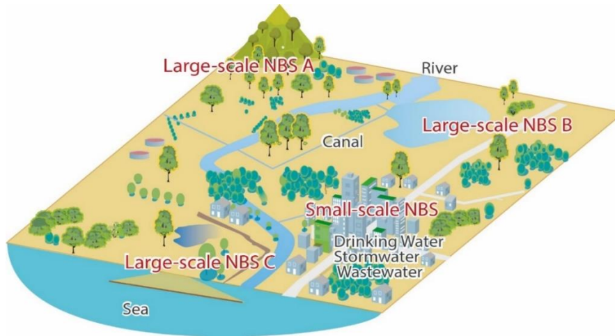
5 Figure 3: Illustration of large and small scale Nature-Based Solutions (NBS); Large-scale NBS A illustrates NBS in mountainous regions (e.g., afforestation, slope stabilization, etc.), Large-scale NBS B illustrates NBS along river corridors (e.g., widening river, retention basins, etc.) and Large-scale NBS C illustrates NBS in coastal regions (e.g., sand dunes, protection dikes/walls, etc.); Typical examples of Small-scale NBS are green roofs, green walls, rain gardens, permeable pavements, swales, bio-retention, etc.
