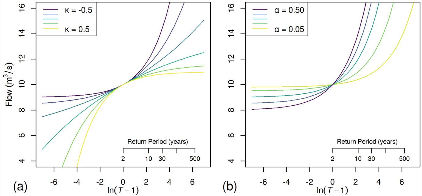
Figure 2: Example GLO flood frequency curves. (a): varying  $\kappa$ , with  $\alpha=0.5$ ,  $\xi=10$ ; (b): varying  $\alpha$  with  $\kappa=0.5$ ,  $\xi=10$ . Plotted on logistic reduced variate scale.
