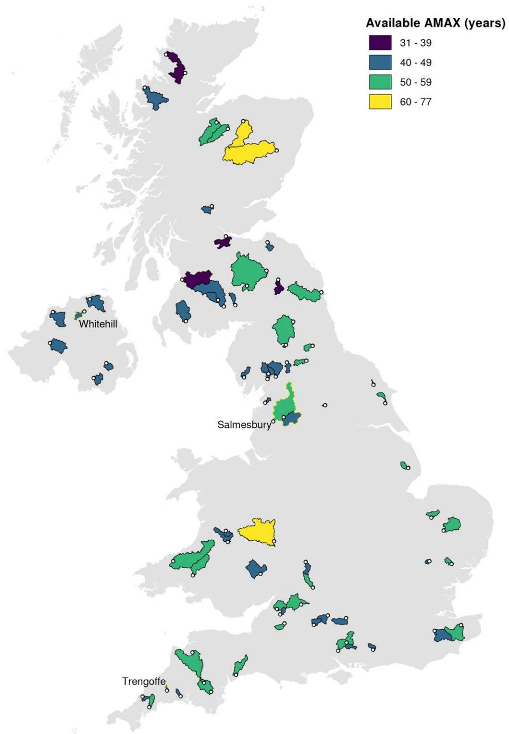
**Figure 1: Locations of the 73 stations used in the analysis, highlighting record length and location of associated watershed. The three stations considered individually in later figures are labelled and outlined in yellow.**
