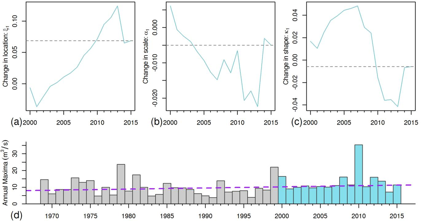
**Figure 8: (a-c) Non-stationary parameters using fixed-start extending windows on the Warleggan at Trengoffe showing change due to addition of single data points,  $\xi_1$ ,  $\alpha_1$  and  $\kappa_1$  plotted. (d) AMAX series highlighting period of extending windows.**
