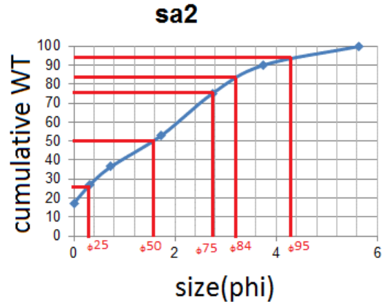
Fig.S17-2 cumulative weight with grain size in Phi unit of core 2 sample no. 2
