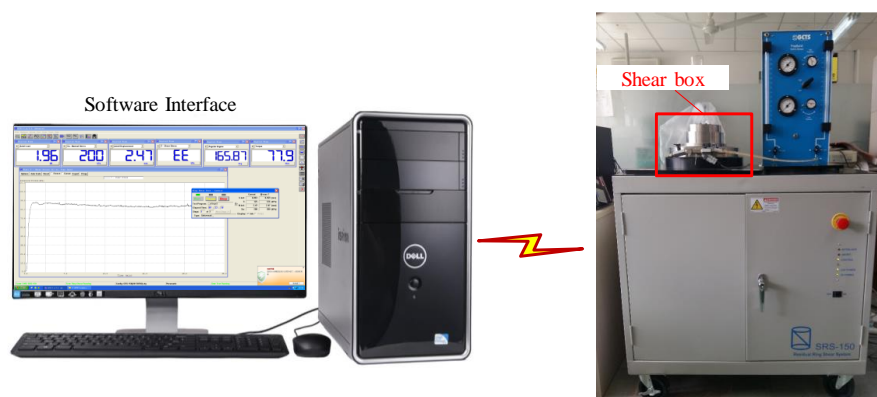
154 155 Fig. 3. Photograph of the GCTS SR-150 Residual Ring Shear testing device and 156 image of the GCTS software interface.
