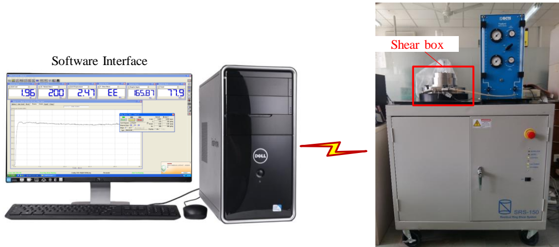
Fig. 3. Photograph of the GCTS SR-150 Residual Ring Shear testing device and an image of the GCTS software interface.
