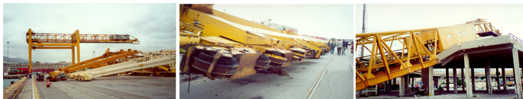
Figure 3: Damages caused by the thunderstorm downburst that occurred in the Port of Genoa (Italy) on 31 August 1994.
