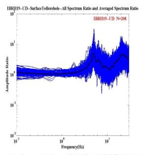
Figture 4. Surface to Borehole Spectral Ratios at IBRH19: (a) EW2/EW1, (b) NS2/NS1, (c) UD2/UD1
