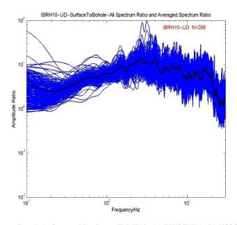
Figture 3. Surface to Borehole Spectral Ratios at IBRH10: (a) EW2/EW1, (b) NS2/NS1, (c) UD2/UD1
