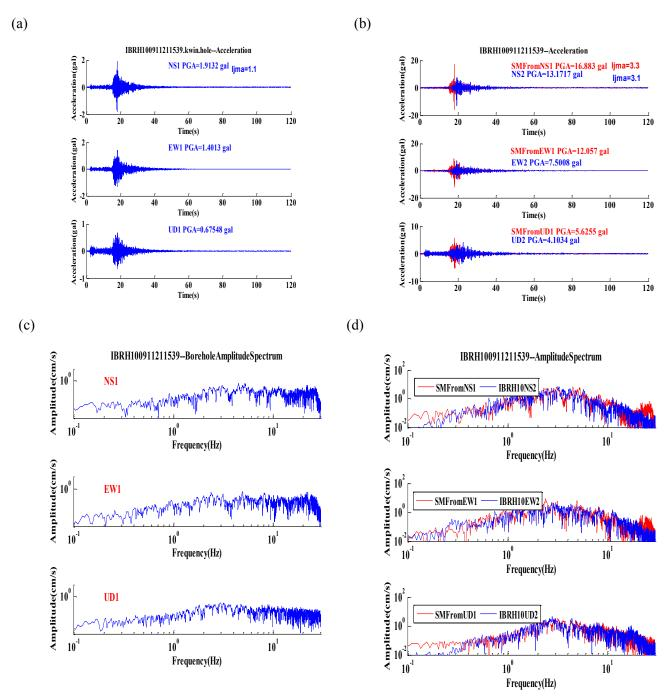
Figture 6. An example of the results of simulation for IBRH100911211539: (a) the observed accertation at the borehole, (b) the observed surface acceleration waveform (blue) compared with the simulated one (red), (c) the spectra of the observed surface record, (d) the spectra of the observed surface record (blue) compared with the simulated one (red).
