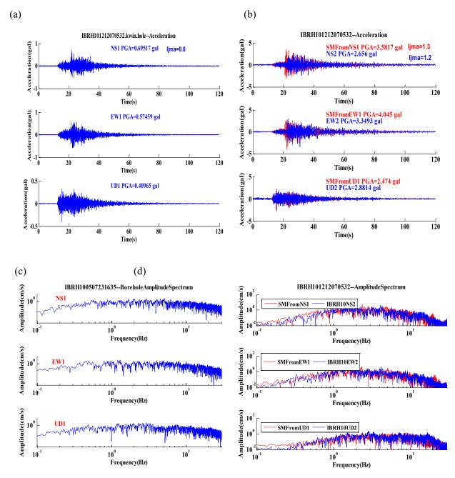
Figture 7. An example of the results of simulation for IBRH101212070532: (a) the observed accertation at the borehole, (b) the observed surface acceleration waveform (blue) compared with the simulated one (red), (c) the spectra of the observed surface record (blue) compared with the simulated one (red).
