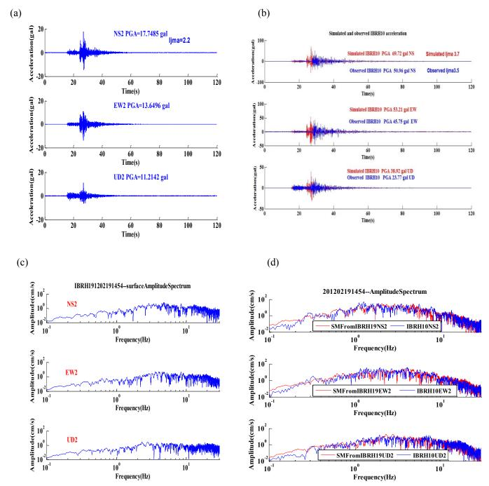
Figure 9. An example of simulation from IBRH19 (surface) to IBRH10 (surface) for the earthquake 201202191454: (a)the observed surface acceleration for IBRH19, (b) the observed surface acceleration waveform (blue) compared with
