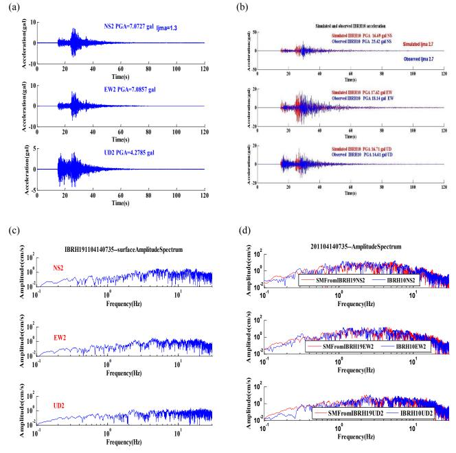
Figure 10. An example of simulation from IBRH19 (surface) to IBRH10 (surface) for the earthquake 201104140735:
