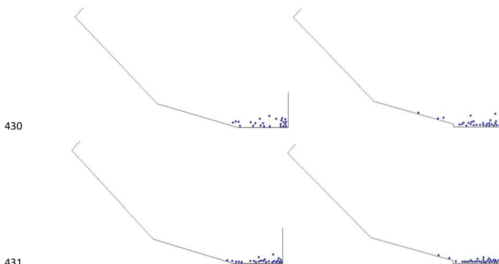
432 Fig. 11a. Flow pattern of blue glass balls 433 flowing along the flume without jump
