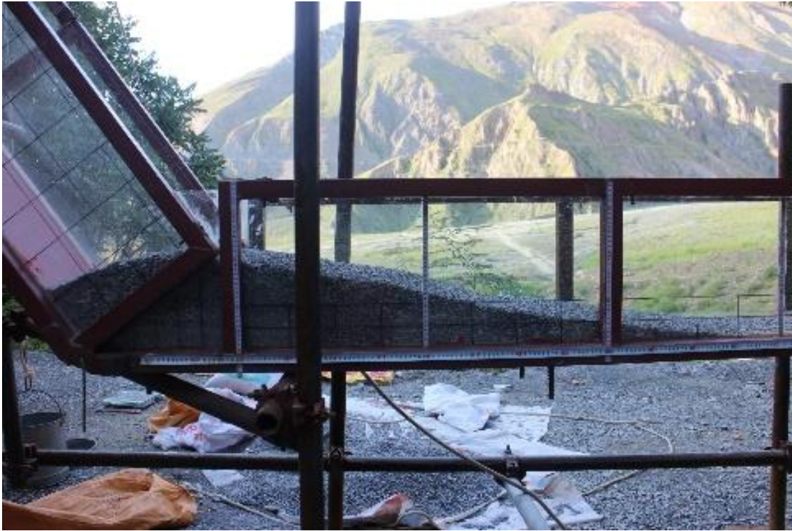
492 Fig.16 Final deposition after the granular flow for two materials (coarse and fine)
