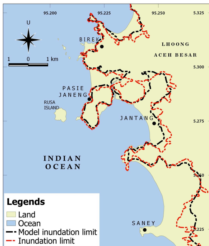
Figure 5: The 2004 tsunami inundation limit at Lhoong based on numerical simulation (black dashed lines) and satellite image digitization (red dashed lines).
