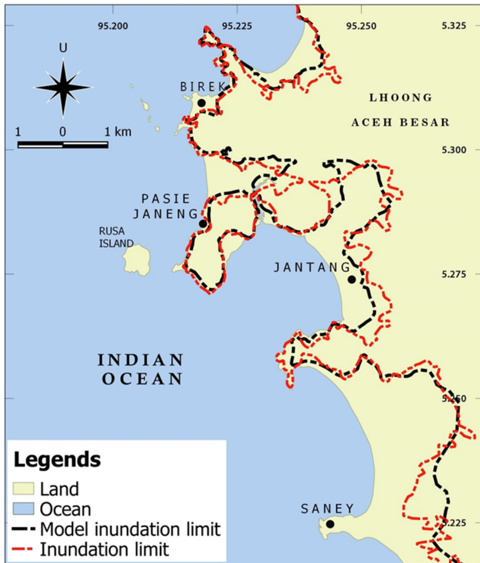
Figure 4: The 2004 tsunami inundation limit at Lhoong based on numerical simulation (black dashed lines) and satellite image digitization (red dashed lines).
