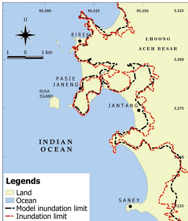
Fig. 3. The 2004 tsunami inundation limit at Lhoong based on numerical simulation (black dashed lines) and satellite image digitization (red dashed lines).
