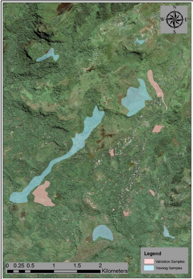
Figure 2 : Landslide failure map catalogue of the Koslanda area with two different training and validating samples
