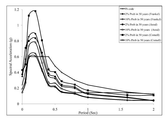
Figure 19 (b): Design spectrum for Patna for 5% damping from 2% and 10% probability of exceedence in 50 years and IS 1893 (2002) at north eastern part of the city (marked in Figure 17 a)
