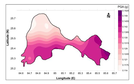
Figure 17 (b): Final seismic hazard map of Patna SSA for 10% probability of exceedence in 50 years using Logic tree approach
