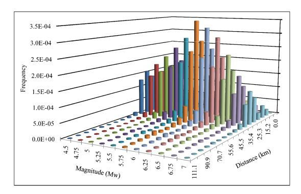
Figure 13 (b): Deaggregation of hazard value at Patna at bed rock at PGA for 10 % probability of exceedence in 50 years using Frankel approach (1995)
