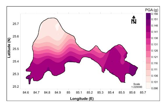
Figure 16 (b): Weighted mean PGA map of Patna SSA for 10% probability of exceedence in 50 years using Frankel approach (1995)
