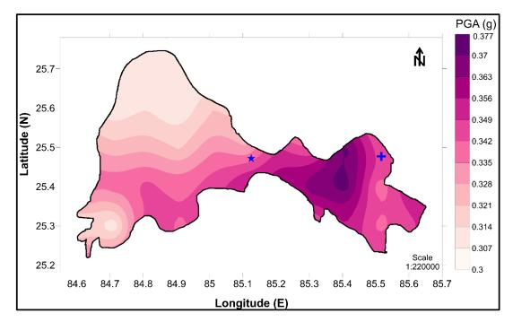
Figure 17 (a): Final seismic hazard map of Patna SSA for 2% probability of exceedence in 50 years using Logic tree approach
