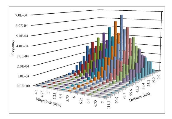
Figure 13 (a): Deaggregation of hazard value at Patna at bed rock at PGA for 2 % probability of exceedence in 50 years using Frankel approach (1995)
