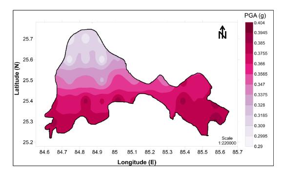
Figure 11 (a): PSHA map for Patna urban centre for 2 % probability of exceedence in 50 years using areal seismic zone
