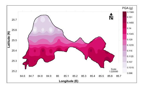
Figure 11 (b): PSHA map for Patna urban centre for 10 % probability of exceedence in 50 years using areal seismic zone
