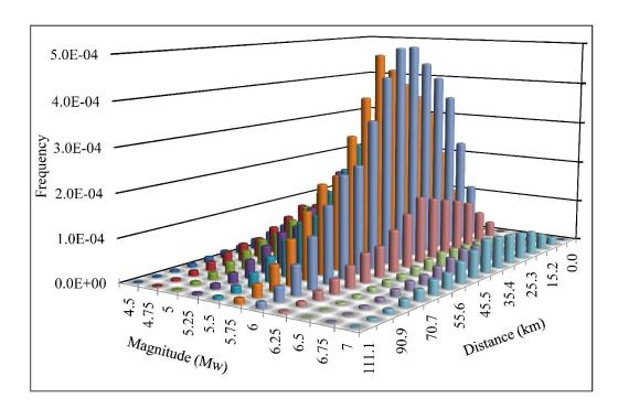
Figure 7 (a): Deaggregation of hazard value at Patna at bed rock at PGA for 2 % probability of exceedence in 50 years using Classical Approach
