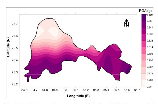
Figure 16 (a): Weighted mean PGA map of Patna SSA for 2% probability of exceedence in 50 years using Frankel approach (1995)
