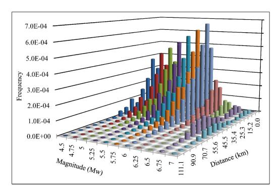
Figure 10 (a): Deaggregation of hazard value at Patna at bed rock at PGA for 2 % probability of exceedence in 50 years using areal seismic zone
