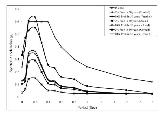
Figure 19 (a): Design spectrum for Patna for 5% damping from 2% and 10% probability of exceedence in 50 years and IS 1893 (2002) at centre of the city (marked in Figure 17 a)
