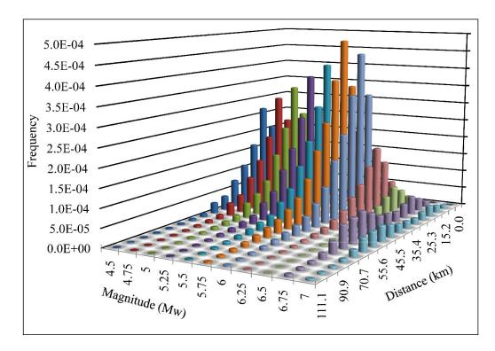
Figure 10 (b): Deaggregation of hazard value at Patna at bed rock at PGA for 10 % probability of exceedence in 50 years using areal seismic zone
