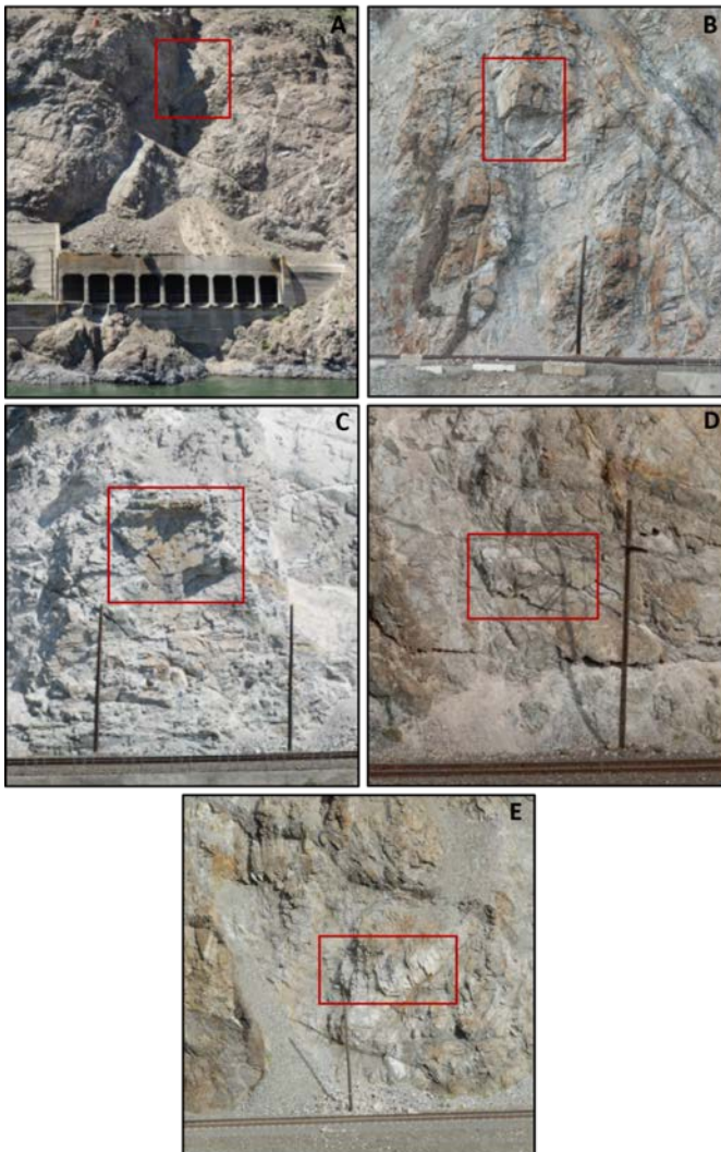
Figure 2: Photos of five rock slope sections, prior to failure, from Goldpan (A) and the White Canyon (B-E) sites adjacent to the CN Railway. The red regions indicate the source zone for the rockfall events discussed in this chapter.
